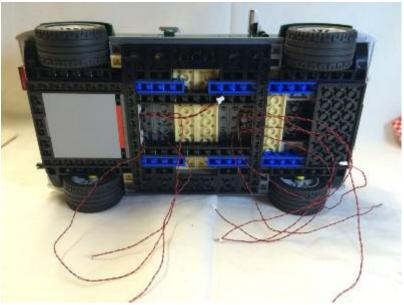
Grab the 12 Port Expansion Board and connect each of the nine wires and the battery pack to the board.
