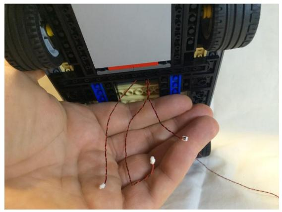
Grab the Coin Cell Battery Pack and feed the plug end of the wires through the same gap.
