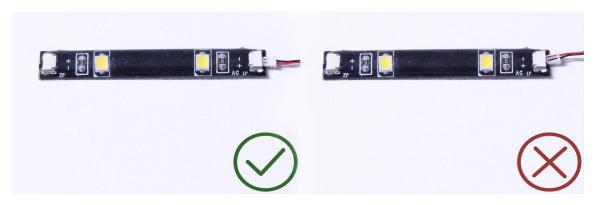
Finally, please pay attention to the positive and negative terminals of the battery when installing the battery case.
