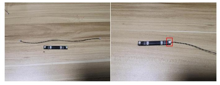
Connect the other end of the connecting cable to the tail of the car as per below.
