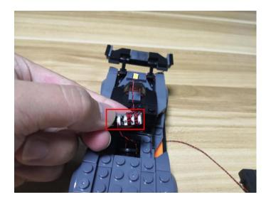
With lighting part facing up, stick the adhesive square to the back of the light.
