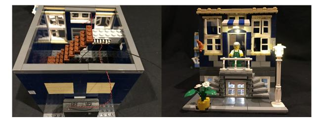
Take another 15cm Connecting Cable and connect it to the next port on the 6-port expansion board. The other end of this cable will be used to connect the left section of this building so set this aside to the left for now.
