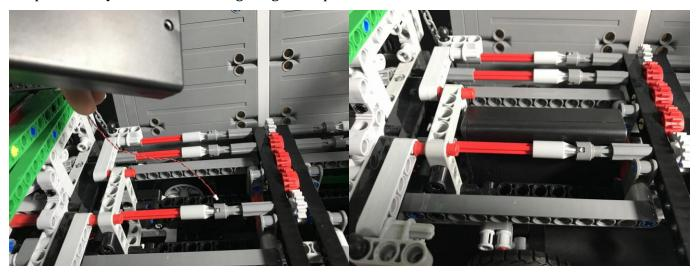
Pass the cable of battery pack toward the expansion board and connect it to the board. And the socket stands on the inner wall of the car
