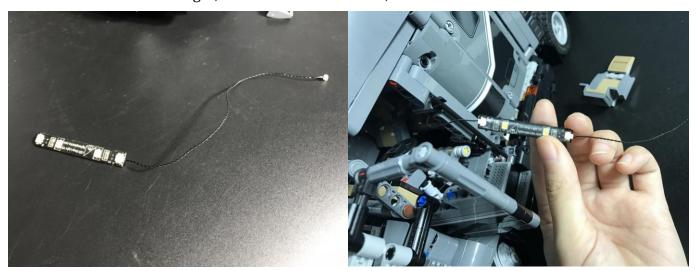
Remove the sticker on the back of the strip light, stick it to the roof, and the 15cm cable is facing the co-pilot direction. Restore the driver's seat.
