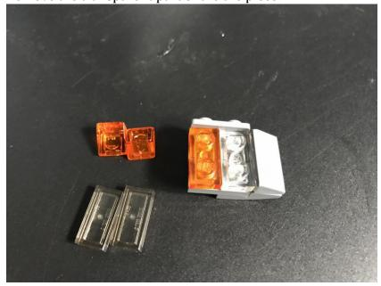
Take the first dot light, put the lighting side up, and fix it with orange transparent piece. Pay attention to the line facing the rear.
