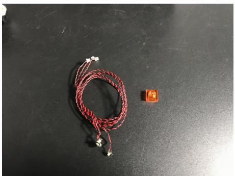
The three dot lights are sequentially fixed with a transparent piece, and the original white transparent piece is replaced with an orange transparent one.
