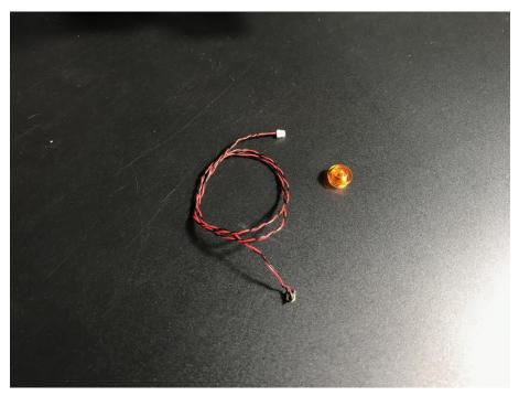
Put the plug end into the gray plug and use the orange transparent small round plate to hold the dot light.
