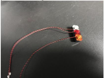
Screw the 3 cables to the left to make a strand, reconnect the taillight.
