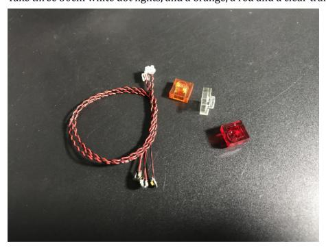
Repeat the previous operation, replace the original transparent piece with the transparent piece provided, and fix 3 dot lights.
