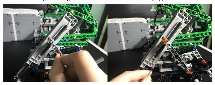
Then insert the plug end into the bottom of the vehicle from the gap next to the yellow brick under the inside of the bracket.
