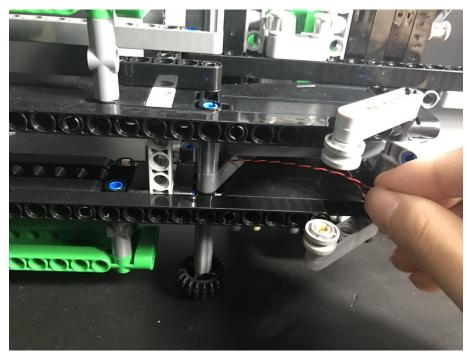
Take a12-port expansion board, connect all plugs, and wrap cables according to the slack of them.
