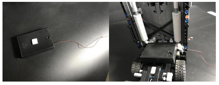
Pass the plug end on the battery pack through the hole in the bottom of the car and pull it toward the front of the car.
