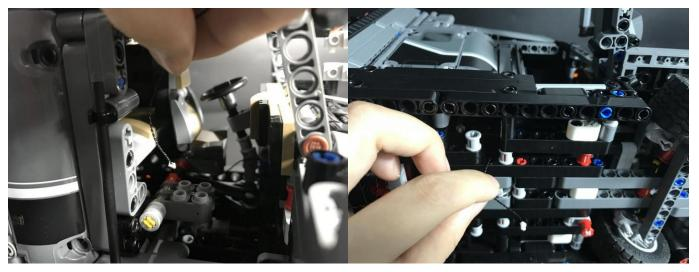
Take the second 12-port expansion board and connect the 15cm cable at the bottom of the car. Connect to the power supply and test it!
