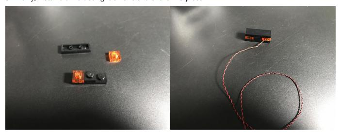
Reconnect the front pieces and twist the 3 cables into one.
