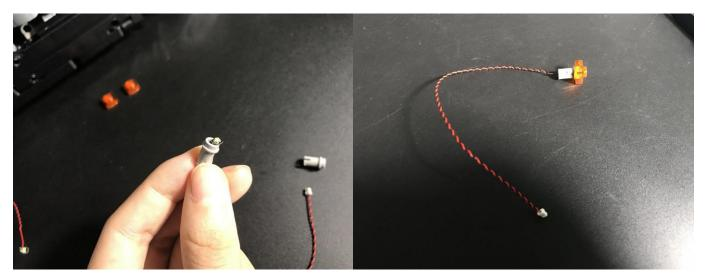
Then insert the plug end from the position where the transparent part was originally installed into the bottom of the vehicle, and fix the gray pin.
