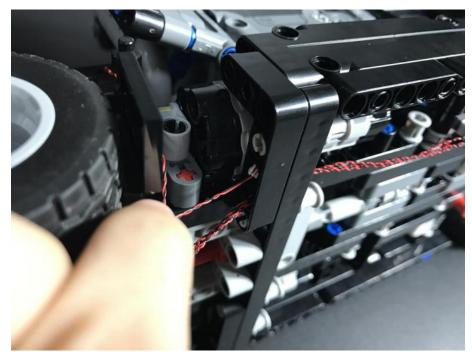
Connect the 12-port expansion board, attach adhesive square to the board, wrap it around the board according to the slack of the cable, and fix the board to the bottom of the vehicle.
