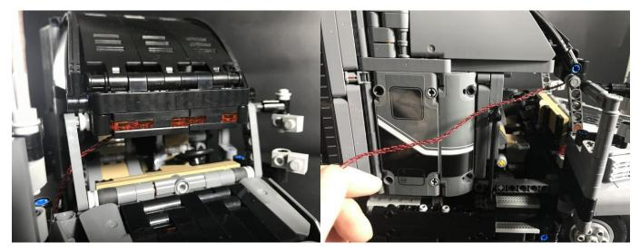
Disassemble the gray plate on the side of the front of the car, pass the cable through the upper beam and then pass it down into the bottom of the car.
