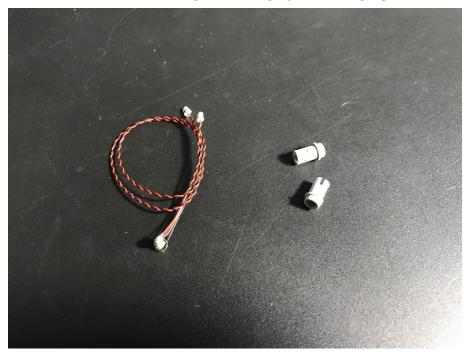
Insert the plug end of the dot light into the gray pin, fold the end of the light into  $90^{\circ}$ , and fasten the lighting side up with a transparent piece.
