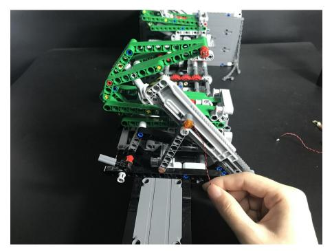
Thread the plug end into the bottom of the car and thread it toward the middle of the car.
