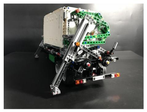
Remove the tail light on the right side and the light transparent piece.
