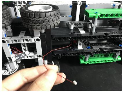
Take 2 gray pins and fix the 12-port expansion board on the hole of the underside technologic piece.
