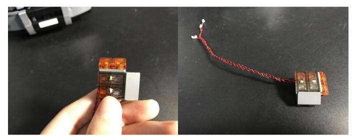
Lift the front cover, pull the cable into the front of the car, and reconnect the headlights.
