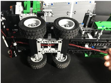
Then remove the orange transparent piece and the gray pin on the rear load-bearing bracket.
