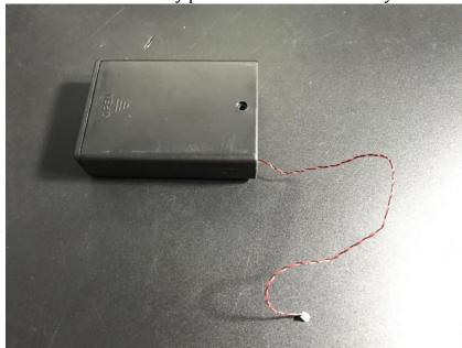
Put the battery pack cable into the bottom of the car, place the battery pack in the space as shown in the picture. Pay attention to the lighting side up.
