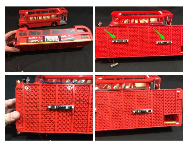
$Take another \, 15 cm \, Connecting \, Cable \, and \, connect it to \, a \, spare \, port \, on \, \, the \, \, 6\text{-port Expansion} \, Board.$
