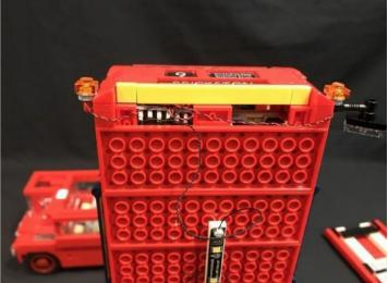
25.) To eliminate excess cable from the 15cm cable between the strip light and expansion board, first remove the next plate underneath and then reconnect over the top as per below
