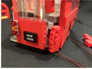
Reconnect the right set of tail lights ensuring the cables are facing toward the left. Fold the cables across the left and then tuck them in behind before reconnecting this section back.
