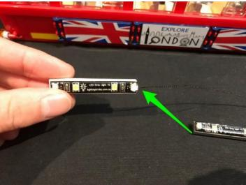
Mount the Strip Light with cable connected to the roof of the Bus in the following position. Thread the other end of the cable across and underneath the grey plates to then connect to the other White Strip Light.
