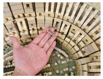
Connect the 50cm connecting cable from the left to the 6-port expansion board at the right.
