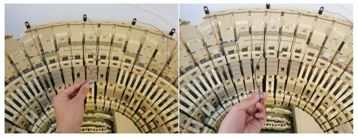
Tuck the expansion board at the following place, place the 50cm connecting cable underneath.
