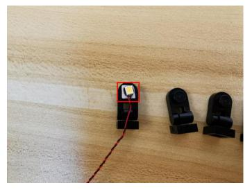
Thread the cable through the gap on the hinge plate.
