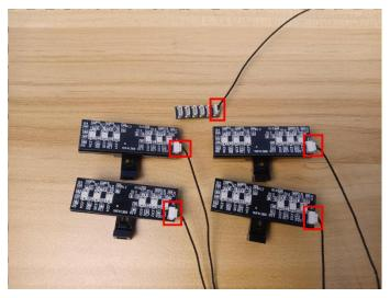
Connect the 3 cables of the background lights to the 6-port expansion board.
