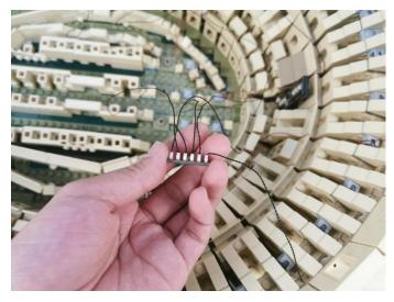
Thread the 50cm connecting cable from the expansion board through to the outside.
