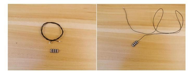
Connect the following 3 cables of the strip lights from the left to the expansion board.
