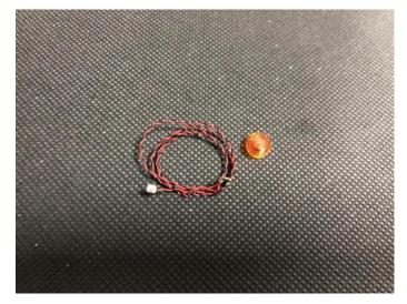
Thread the cable through the pin, pull the cable out till the light is placed inside, secure the light with the trans orange plate.
