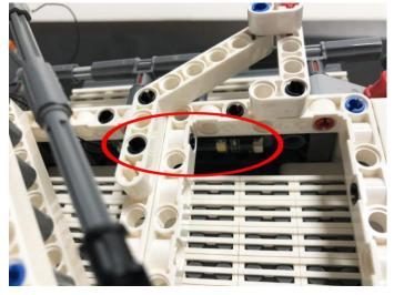
Place the connecting cable from the strip light as per below, pull it toward the 12-port expansion board.
