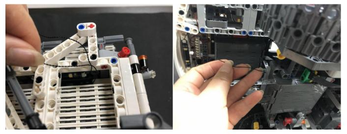
Pull the cable out from the following hole (you can pull it out from any hole).
