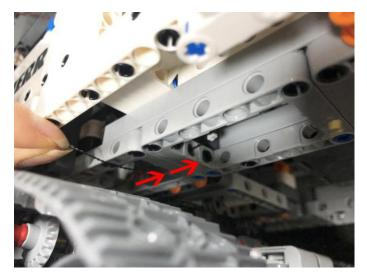
Continue to place the cable as per below, pull the cable to the back of the battery pack.
