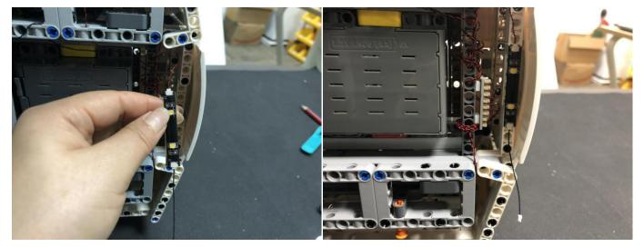
Connect the connecting cable from the strip light to the expansion board asper below.
