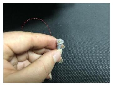
Thread the cable through the following black piece, reconnect the trans piece.
