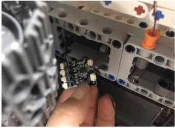
Reconnect the Remote Control Switch Board.
