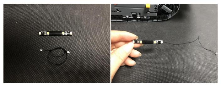
Stick the strip light to the roof of the control cabin. Pull the cable backward.
