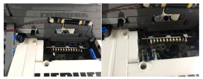
Repeat the steps above to install the other light, thread the cable through the space next to the wall, and connect the cable to the expansion board.
