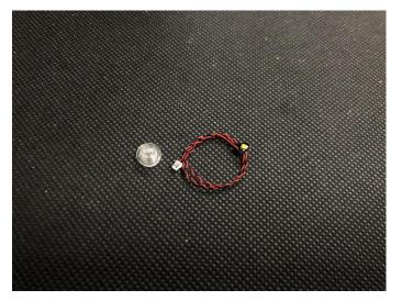
Thread the cable through the pin, pull the cable out till the light is placed inside, secure the light with the trans round plate.
