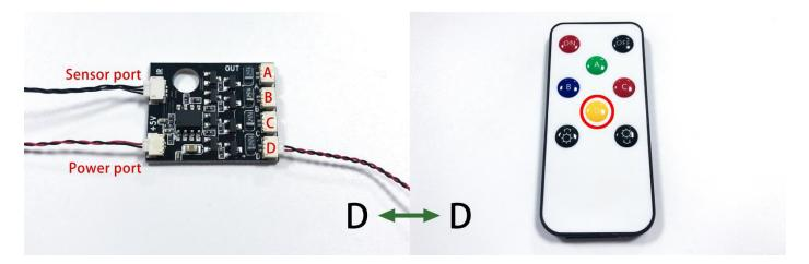
With connecting cable side facing down, connect the cable to the bigger port on the remote control
