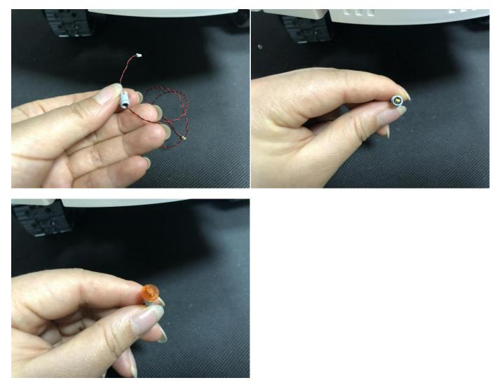
Thread the able through the following black piece, reconnect the piece we removed before.
