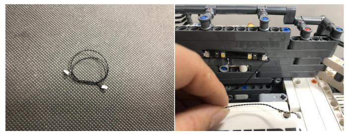
Take a 12-port expansion board, connect the connecting cable to it.
