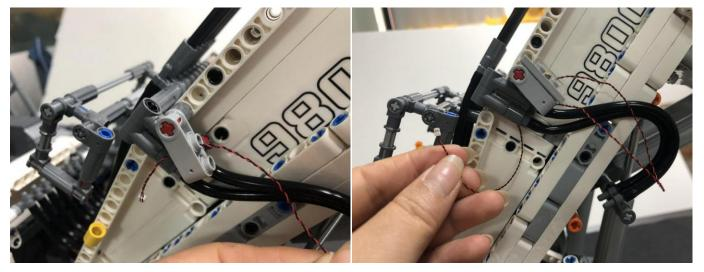
Pull the cable downward from the inner side, in case of interfering the excavator, do not thread the cable through any holes.
