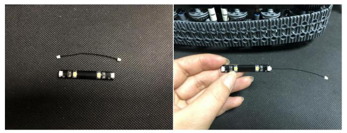
Connect the cable of the light to the strip light, stick the strip light to the following place.
