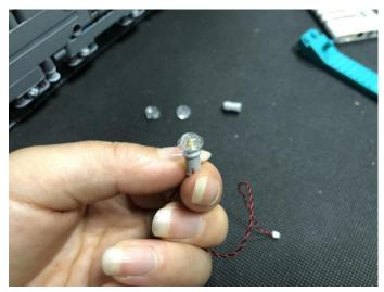
Lift the gray piece a bit (to help the cable thread through), thread the cable through the hole.
