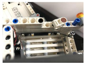
Thread the cable through the following space, and connect it to the expansion
