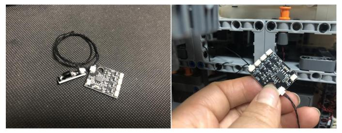
Stick the Remote Control Switch Board to the following place with adhesive squares.
