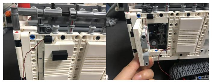
Thread the cable through the space near the doorframe to the bottom.
