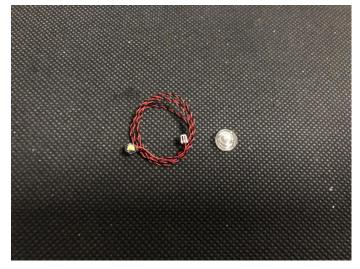
Thread the cable through the pin, pull the cable out till the light is placed inside.
