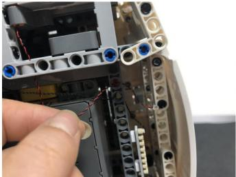
Tuck excess cable before connect it to the expansion board.
