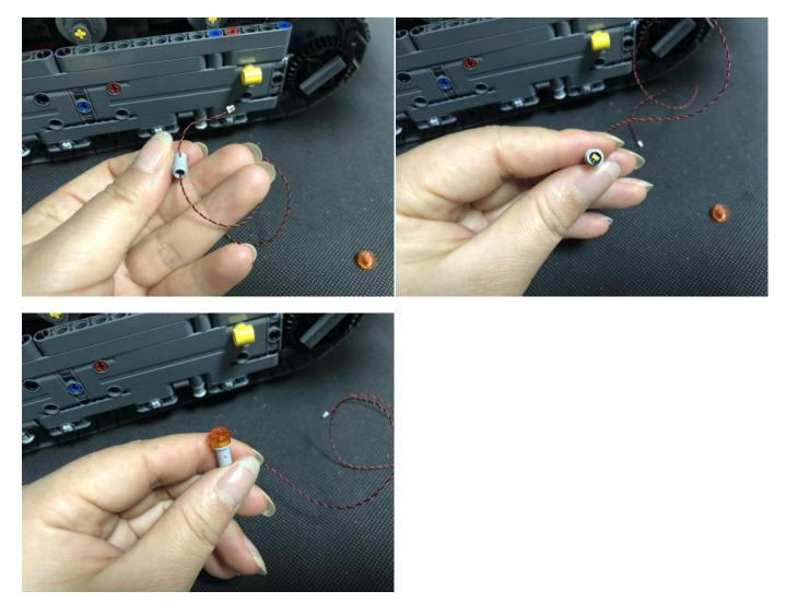
Thread the cable through the following spaces, reconnect the pieces we removed before.
