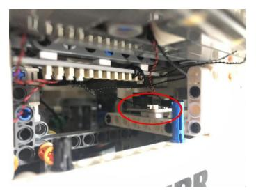
Turn the excavator to its side, pull the cable from the Multi Effects Board out.
