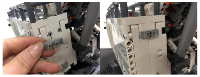
Pull the cable out from the bottom, place it alongside the car to the back.
