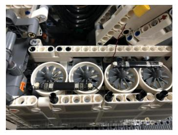
Thread the cable through the following space, pull the cable out from the bottom.
