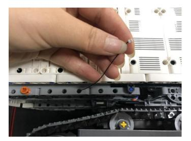
Take a 6-port expansion board, connect the connecting cable to the expansion board.
