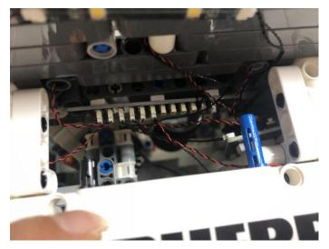
Take a 30cm connecting cable, connect it to the expansion board.
