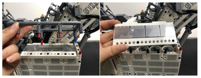
Continue to install light for the following trans piece, remove the piece and disassemble it.
