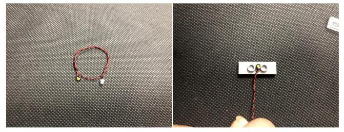
Reconnect the trans piece to secure the light, thread the cable through the following space.
