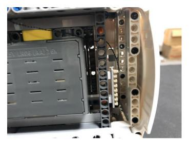
Take a warm white strip light, a 15cm connecting cable, connect the connecting cable to the strip light.
