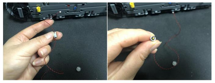
Secure the light with trans round plate, continue to thread the cable through the following black piece, reconnect the pin.
