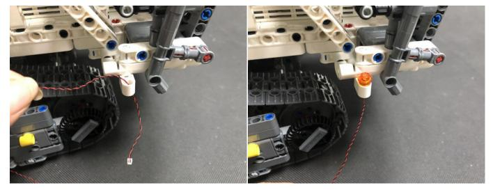
Turn the excavator to its side, thread the cable through the orange piece, and continue to thread it through the following spaces.
