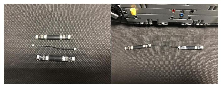
Connect the cable from the light to the strip light, stick the strip light to the following place.
