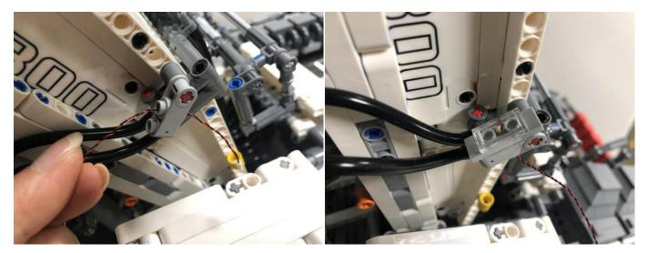
Thread the cable to the inner side, pull it downward, in case of interfering the excavator, do not thread the cable through any holes.
