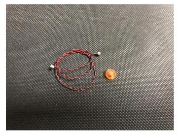
Thread the cable through the pin, pull the cable till the light is placed inside, secure the light with trans orange plate.
