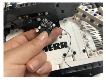
Stick the Multi Effects Board to the following place with adhesive squares. Thread the cable to the bottom.
