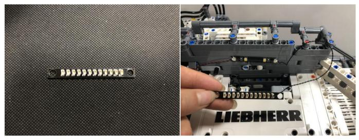
Stick the expansion board to the following place, remove the following piece.
