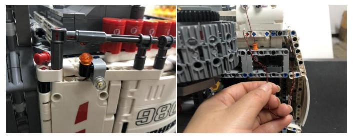
Wind excess cable around the following piece before connect it to the 8-port expansion board.
