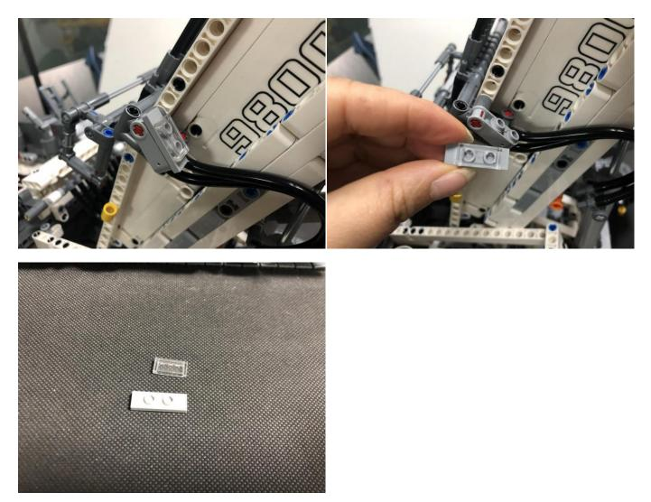
Take a warm white 30cm dot light, place the light between the 2 studs, secure the light with trans piece.
