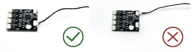
Connect the other end of the connecting cable to the sensor.
