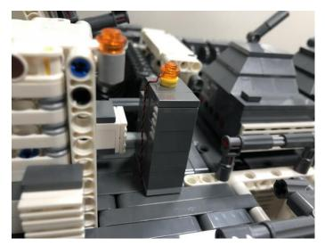
Turn the car over to its side, connect the cable of the light to the expansion board as per below.
