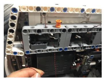
Tuck excess cable before connect it to the 8-port expansion board.
