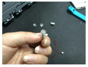
Lift the gray piece a lit (to help the cable thread through), thread the cable through the hole.
