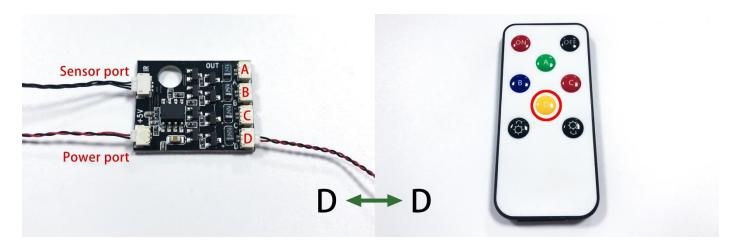
With connecting cable side facing down, connect the cable to the bigger port on the remote control board as per below.
