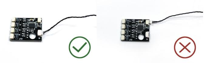
Connect the other end of the connecting cable to the sensor.
