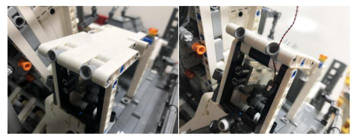
Reconnect the pin, pull the cable backward as per below.
