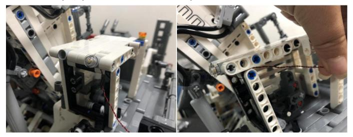
Remove the seat, thread the cable through the space underneath.
