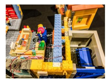
28.) Take the 2 cables from the flashgame#1 and 2 and pull them up towards the other end of the store. Take another 30cm cable and lay the cable along side the other 2 cables. Leave about 3cm of free cable sticking out the front. This will be used to connect to striplight#3 later.
