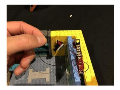
19.) We can test our current lighting circuit as you go by simply turning on the battery pack. This is a good idea as you want to ensure all is working before you connect back bricks into original positions. Let's turn it on to see how it looks so far.
