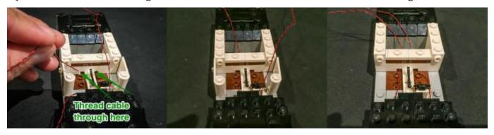
Ensure the cables are laid on the side of each of the brown Lego studs 6.) Start securing the cables down by reconnecting back Lego plates and tiles over the top. Before doing so, ensure that the cables are laid in between studs exactly the same way as the below images.
