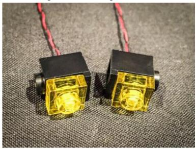
3.) Reconnect the 2 head lights back to the front of the car ensuring the cables for the lights are facing up.
