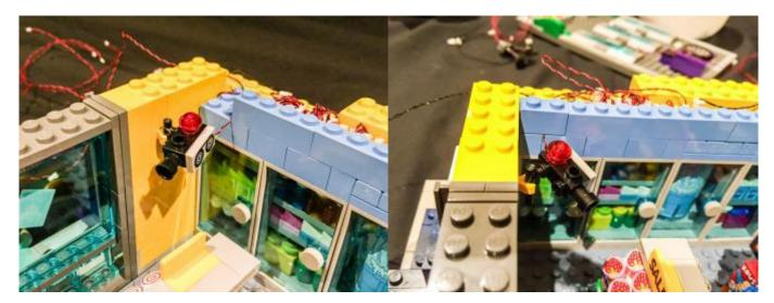
Ensure cables are laid in between studs before connecting bricks over them.
