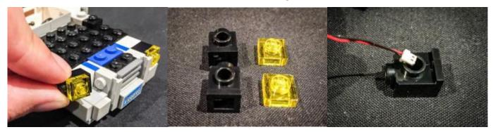
Pull the cable from the back of the black brick all the way until the LED component is flat up against the other side of the brick. Ensure that the LED component part is facing the correct way up, then secure this down by reconnecting the transparent yellow Lego plate over the top.
