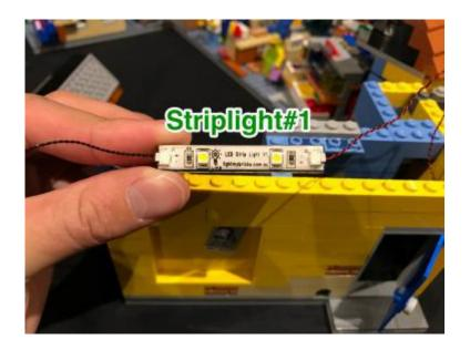
Take the roof of this section and flip it over then connect/stick the strip light in the following position. Ensure that you loop the 30cm cable above and then underneath the strip light so that it is not visible from the inside of the store.
