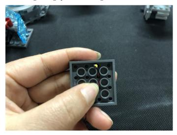
Reconnect the roof. Fixed lamp (note: pull the cable out from the back)
