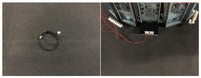
Take a USB power cable, connect it to the expansion board, then, connect the other end to the power source
