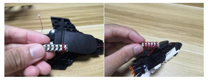
Stick the last 2 adhesive squares to the back of the expansion board, stick the expansion board to the battery pack as per below.
