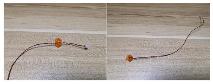
With lighting part facing up, place the cable at the opening of the round plate as per below.
