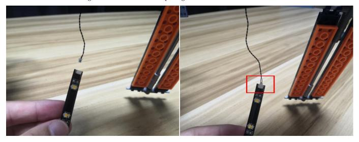
Stick the strip light to the following place on the solar panel, pull the 30cm connecting cable down, reconnect the solar panel.
