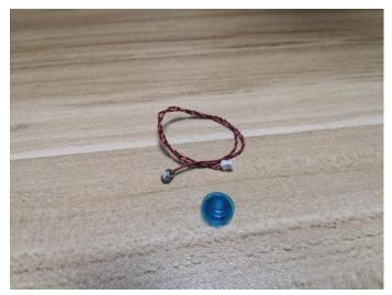
Place the light inside the round plate (with lighting part facing down), stuck the cable at the opening on the round plate as per below.
