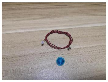
Thread the cable through the following hole, pull the cable out, keep the lighting part facing outside.
