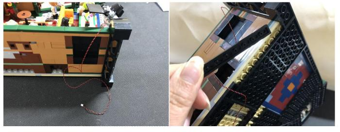
Pull the cable to the bottom, reconnect the piece we removed before to secure the cable, then, connect the cable to the expansion board#2
