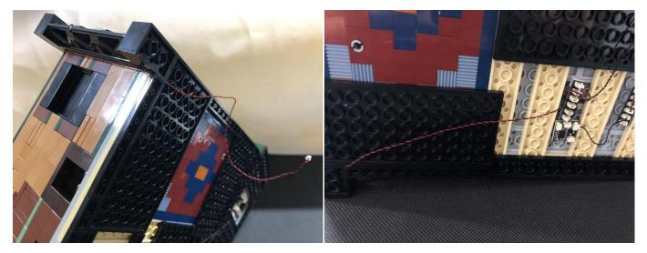
Take a 5 cm connecting cable, assemble the expansion board #2 and the Flicker Effects Board together with the 5 cm connecting cable
