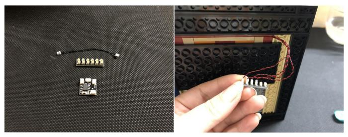
Connect the expansion board and the Flicker Effects Board together with the 5cm connecting cable. (note: do not connect the cable to the power port on the Flicker Effects Board)
