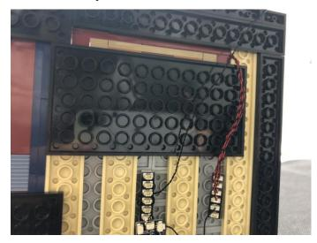
Connect the cable from the other spotlight to the expansion board. Turn the house to its side, remove the following piece
