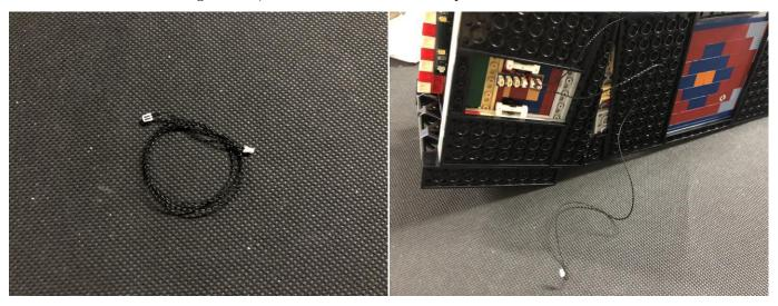
Connect the other end of the cable to the output port on the flicker effect board, secure the cable with a 1x6 plate (the colour depends on the package)
