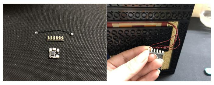
Connect the expansion board and the Flicker Effects Board together with the 5cm connecting cable. (note: do not connect the cable to the power port on the Flicker Effects Board). Stick the expansion board and the flicker effect board to the bottom with adhesive squares.
