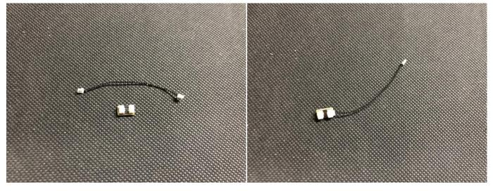
Connect the cable from the spotlight to the 2-port expansion board as per below, and connect the other end of the 5cm connecting cable to the expansion board #2
