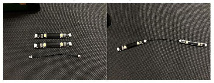
Connect the cable from the spotlight to the strip light, and place the cable as per below
