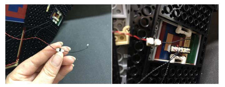
Take the USB cable, connect it to the expansion board#2, as per below
