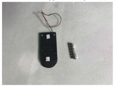
Connect all the cables to the expansion board, tuck the excess cables around the expansion board, stick the expansion board and the battery pack at the bottom of the train
