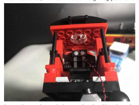
Remove the gray plate inside the train, place the cable underneath it
