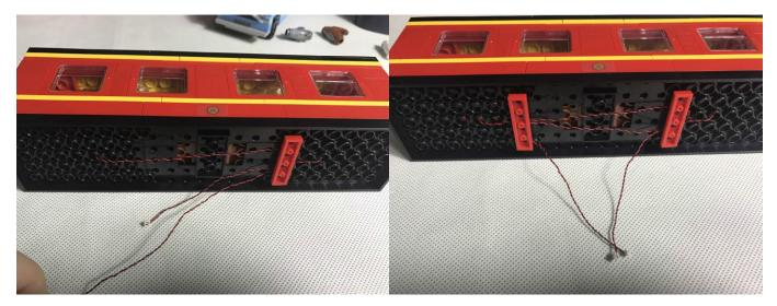
Take the Flat Battery Pack, inserted with batteries, a 6-port expansion board, then, stick adhesive tapes at their backs
