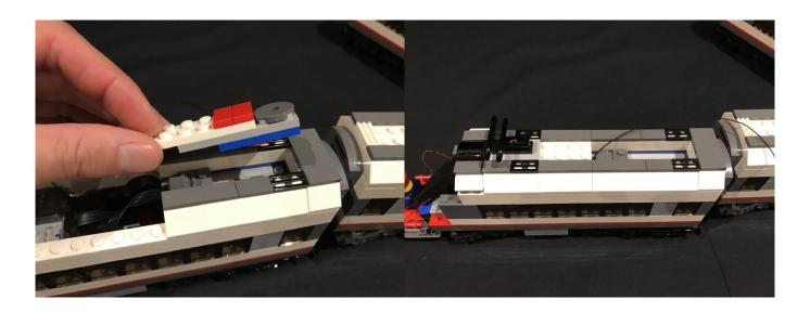
12.) Remove the following section from the back of this carriage and then bring the cable across to the next carriage. Reconnect the section over the cable ensuring the cable is laid in between studs.
