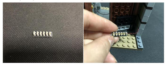
Stick the expansion board to the back of the door with adhesive square.
