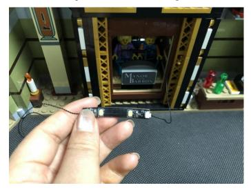
Stick the strip light over the following frame, tuck excess cable as per below.
