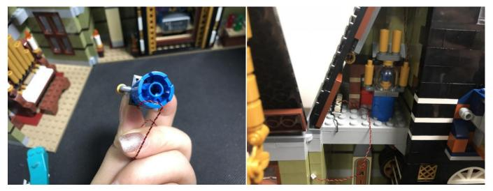
Tuck excess cable before connecting it to the expansion board, stick the expansion board to the following place.
