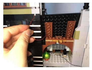
Lift the gray plate, thread the cable through the following space to the expansion board.
