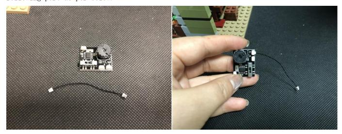
Connect the other end of the connecting cable to the expansion board.
