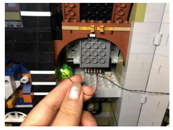
Reconnect the gray plate, tuck excess cable before connecting it to the expansion board.
