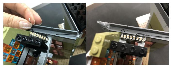
Take a white strip light, a 5cm connecting cable, connect the connecting cable to the strip light.
