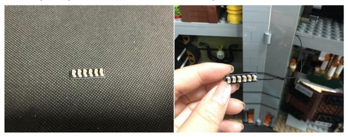
Tuck excess cable before sticking the expansion board to the following place.
