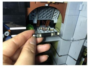
Create a gap between the following pieces, thread the strip light through the gap as per below.
