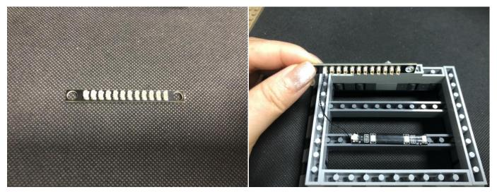
Stick the expansion board to the following place with adhesive squares, reconnect this part as per below.
