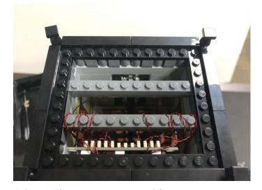
Take a 50cm connecting cable, connect it to the 12-port expansion board.
