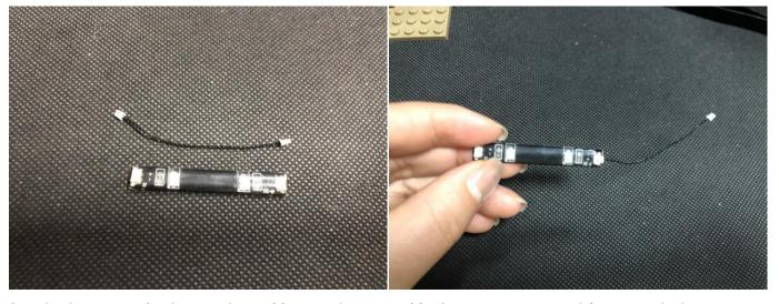
Stick the strip light to the following beam, pull the connecting cable toward the expansion board.
