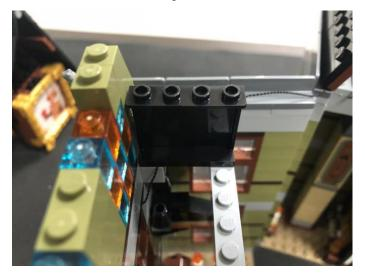
Take a green strip light, a 5cm connecting cable, connect the connecting cable to the strip light.
