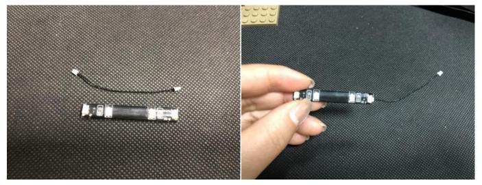
Stick the strip light to the following place, pull the cable out and pull it toward the expansion board.
