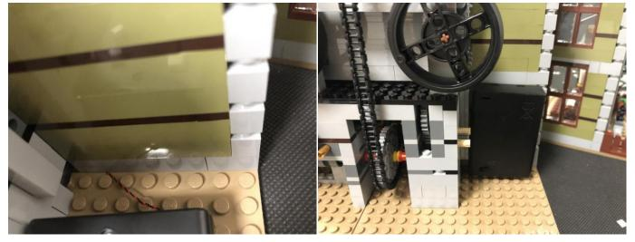
Connect the connecting cable from the battery pack to the expansion board, tuck excess cable as per below.
