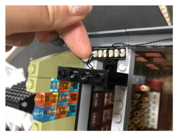
Take a white strip light, a 15cm connecting cable, connect the connecting cable to the strip light as per below.
