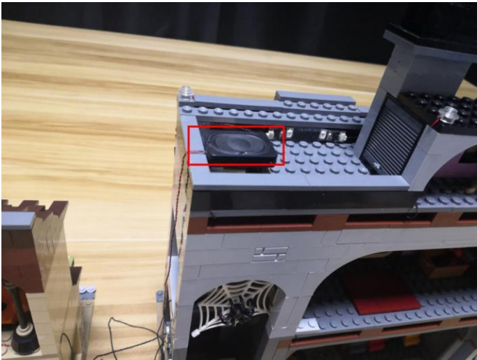
Stick adhesive squares on the audio device, stick it on the roof.
