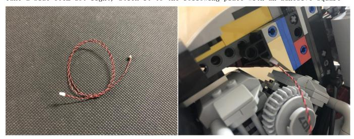
Thread the cable through the gap behind the gray wheel
