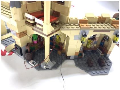
Take a 6-port expansion board, a USB power cable. Stick adhesive tapes to the expansion board
