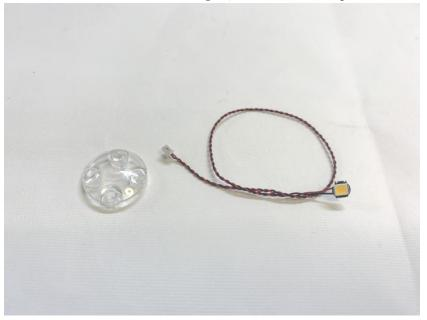
With lighting part facing down, secure the light underneath the roof with the round plate
