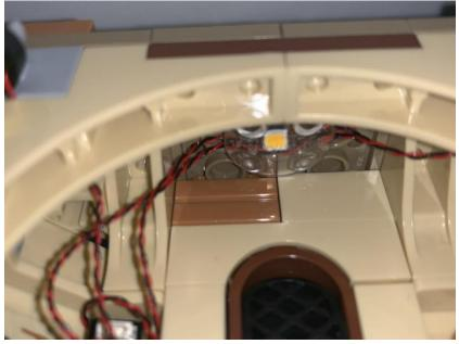
Thread the 15cm connecting cable from the expansion board through the gap on the wall
