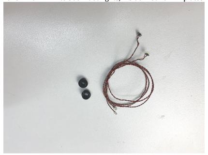
Thread the connector of the light through the hole on the black plate, pull the cable till the lighting side is facing up. Connect the black round plate and the yellow round plate over the light
