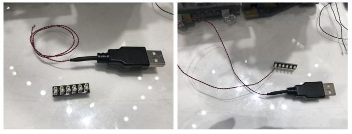
Take 2 adhesive squares and stick them on both ends of the board. Connect the 4 cables to the 6-port expansion board and wrap them around the board.
