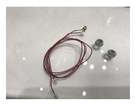
Take one of the 30cm warm white lamp dots, pull the plug end out from the side of the black large round hole, and turn the lamp face up.
