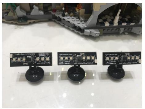
Connect the 50cm cable and the two 30cm cables to the input ports of the three atmosphere lights, and the other end to the 6-seat socket.
