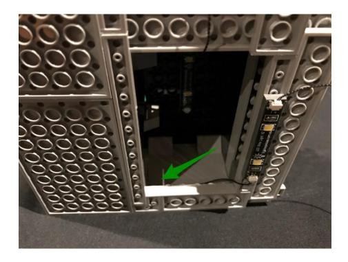
29.) Place the Battery Pack on top of the roof in the below position ensuring the ON/OFF switch is facing up.
