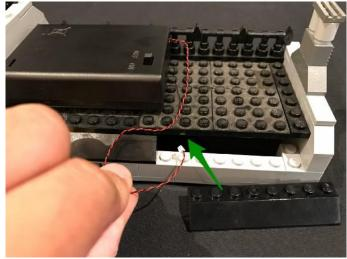
Pull the cable through from the inside of the roof and then connect it to the spare port on striplight#6
