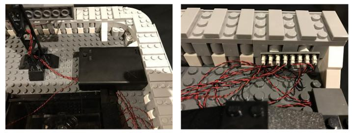
You can secure the battery pack a little more and to prevent it from moving around by connecting a Lego piece on the top side of the battery pack.
