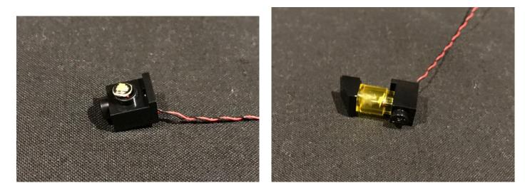
8.) Reattach the lamp with Dot Light installed onto the pillar ensuring the cable is laid in between the 2 black Lego studs, then reconnect the top two layers of the pillar.
