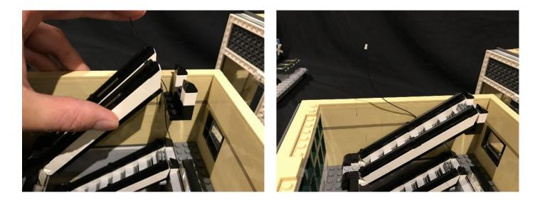
22.) Take the entire third level and then pop it onto its side. Take another two strip lights (striplight#3 and #4) and connect/stick them in the following positions. Connect a 5cm cable in between the strip lights and take a 30cm cable and connect it to the right port of striplight#3. All shown below.
