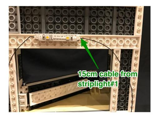
21.) Hide the 15cm cable underneath the white Lego plate and then thread the other end of the 30cm cable up to the next floor above. Connect back the second level and then pull up the 30cm cable from underneath.
