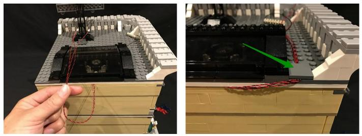
33.) Connect the cables from the chandelier to the next available ports on the 8-port expansion board and then secure the expansion board to the inside of the roof's edge using 2x self adhesive squares. Neatly lay the cables down below.
