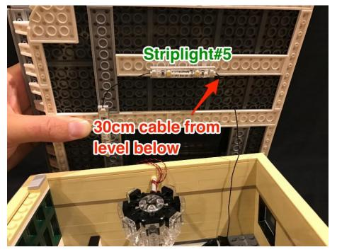
32.) Take the 3 cables from the chandelier and then pull them to the right and then up across the roof of the building. Lay them down neatly and secure them down using any spare Lego plate or brick you might have, ensuring the cables are in between the studs.
