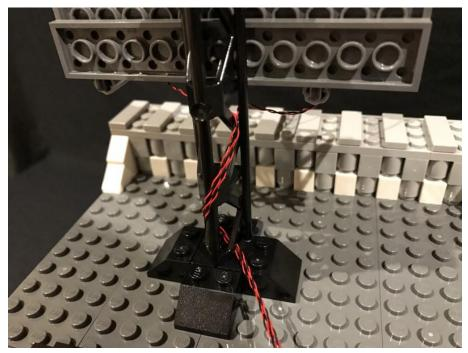
36.) Connect all three cables into the next available ports on the 8-port expansion board and then neatly lay the cables down as per below.
