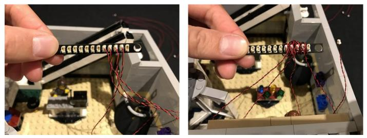
Take the cable from lamp post and connect this into the far right port of the expansion board.
