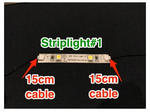
Stick the strip light underneath the centre of the roof in the following position and then thread both cables up in between the doors and ceiling. Pull them up from inside of the building.
