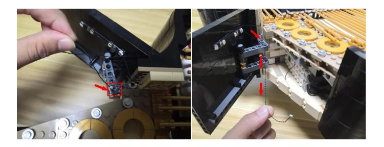
Take a 6-port expansion board, connect the cable we threaded before to it, connect the following 5cm connecting cable to it.
