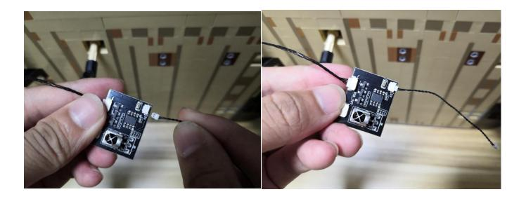
Stick the RGB Remote Control Switch Board to the following place (tighten the cable up).
