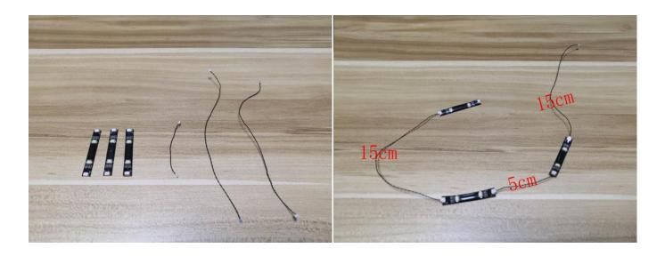
Connect the cable from the corner to the following strip light.
