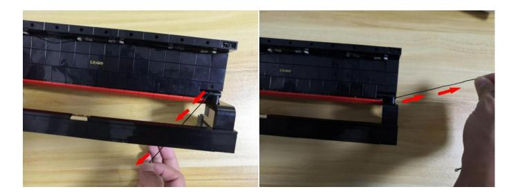
Thread the cable through the following space underneath the piano.
