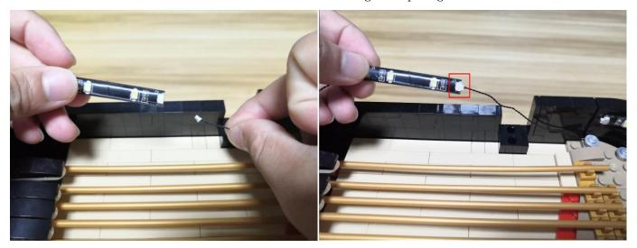
Stick the strip light at the following place, thread the cable and the strip light through the following space.
