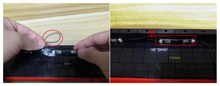
Stick the third strip light at the right side as per below, wind excess cable and press it underneath the strip light.
