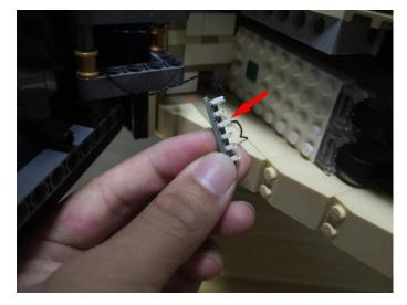
Take a AAA battery pack, connect it to the expansion board, and place the battery pack at the following place.
