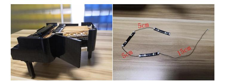
${\tt Connect\ the\ 15cm\ connecting\ cable\ underneath\ the\ piano\ to\ the\ white\ strip\ light\ as\ per\ below.}$
