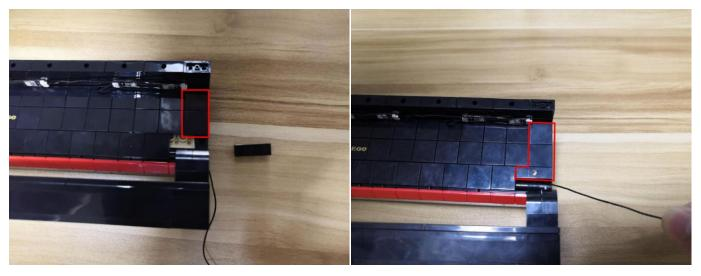
Pull the cable out behind the following plate.
