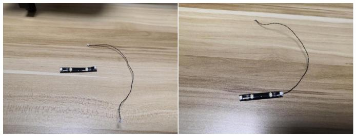
Connect the 15cm connecting cable underneath the music stand to the strip light, stick the strip light to the following place, pull the cable leftward.
