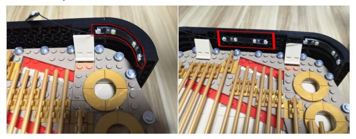
Stick the third strip light at the arc corner, tuck the cable as per below.
