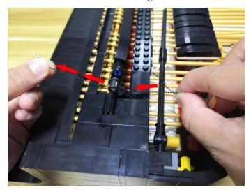
Take a white strip light, a 15cm connecting cable, connect the connecting cable to the strip light.
