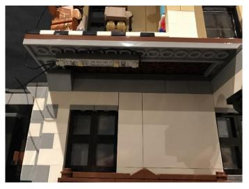
19.) Hide the excess from the 30 cm cable by laying parts of the cable underneath the dark grey tiles as pictured below. Ensure you leave enough cable for this section to open the whole way.
