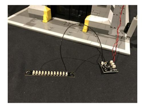
Take 4x adhesive squares and stick 2 to each board. Mount the traffic light board to the inside of the building in the top right corner. Hide the excess cables from the traffic light underneath the board.
