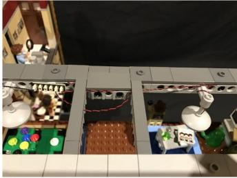
41.) We will now install a light to the window lamp. First remove this lamp as well as 2x2 brick underneath. Install another Dot Light to this lamp following the same process as the bedside lamp in step 27.
