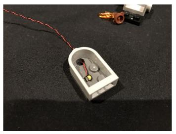
Secure the Dot Light in place by reconnecting the fire piece directly over the top, then reconnect the pieces of the fire place. Reconnect the chimney with light installed to original location.
