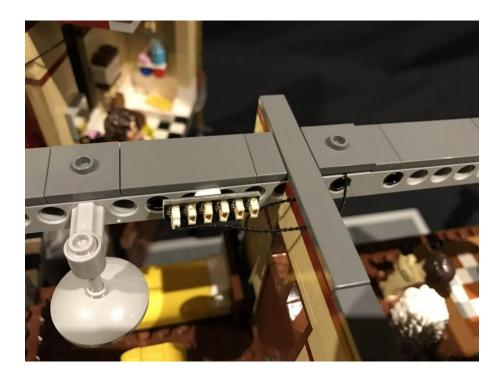
27.) We will now install a Dot Light to the bedroom lamp. Start by removing the lamp as well as drawers underneath, then remove the lamp shade.
