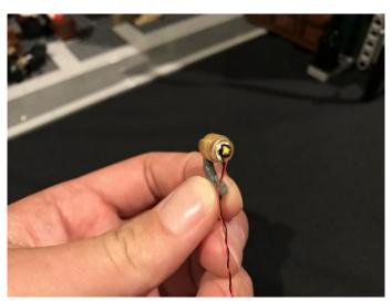
Thread the connector end of the Dot Light cable through hole of the grey base before reconnecting the lamp to it.
