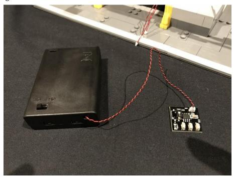
Ensure the effect switch is at the label "3". (The other option "2" is for a 2-light traffic lights effect which we don't for this)
