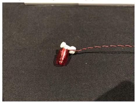
Thread the connector end through the front hole of the light grey brick and then out through the base. Pull this all the way through until you can connect the grey tap piece to the grey brick.
