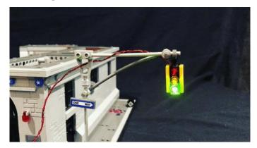
7.) We can now remove the battery pack cable from the top traffic light board (as we only connected this to test the traffic light board). Replace this with a 15cm connecting cable, then connect the other end to the first port on the 12-port expansion board
