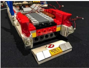
Remove the transparent red cone pieces from each side of the car. Take a standard Dot Light(non kashing) and place it over the top of the red stud on the side of the car ensuring the LED component part is facing the correct way up. Secure the LED in place by reconnecting the transparent red piece over the top of it. Ensure the cable from the LED is facing toward the middle so that we can hide it behind the back piece we removed earlier.
