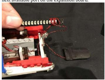
14.) Connect the cables from the front lights into the next available ports of the expansion board then tuck the cabling underneath the expansion board in the back seat section of the car.
