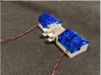
17.) We will now install kasing LEDs to the blue spot lights at the front. Remove the grey plates with clips from the pole and then disconnect the round blue pieces from them.
