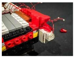
Repeat this step for the tail light on the other side using another standard Dot Light. Reconnect the back piece with the ghostbusters logo on it and ensure the cables from the LEDs are hidden behind.
