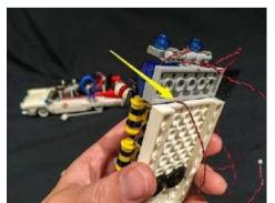
19.) Take all the cables and lay them down the middle of the middle white plate before reconnecting the back white plate underneath.
