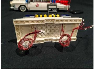
29.) Take another expansion board (expansion board#2) and connect the first group of 6 lights from the front section of the roof to the first available ports on the expansion board.
