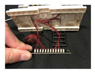
30.) Take the 5cm connecting cable from the kit and connect it to the last available port on expansion board#2.
