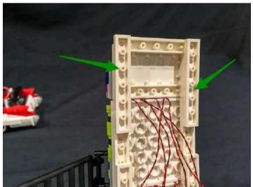
27.) Turn the roof on its side to allow you to then group all the cables from the front roof LEDs.
