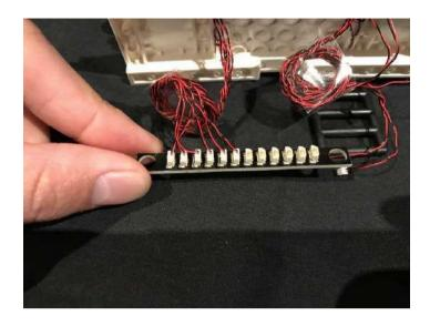
Connect the other group of lights from the back section of the roof to the next available ports on the expansion board#2.
