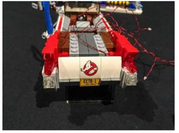
11.) It's time to neaten up all the cabling from the LEDs we have installed so far. Take the 5 cables from the front lights and twist/wind them around each other starting from the base working your way up. They should all come together neatly.
