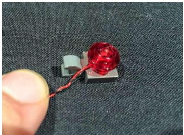
Ensure the cable from the LED is facing the same way the clip underneath is facing Reconnect the round grey Lego piece to another provided Lego piece with clip then re-attach the 2 pieces back to the pole before then reconnecting this back to the roof. Ensure that the cable from the red LED is hidden behind the pole.
