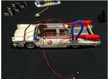
12.) Connect the cables from the tail lights into one of the 12-port expansion boards (expansion board#1) by first winding them around the board before connecting them into the first 2 available ports. We are winding them around the board so that we don't have too much excess cabling to have to hide later on.
