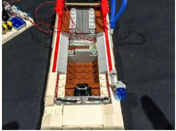
10.) We will now install 2 LEDs to the tail lights. Turn the car to the back and remove the back window and white back section of the car. The back section should remove in one piece.
