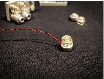
Install the remaining LEDs to all front headlights (2 on each side) using the above process so that we have a total of 4 standard Dot Lights installed. Reconnect the light pieces back to the 2 Lego 2x4 plates ensuring that the cables from the LEDs are facing upward and then reconnect the plates back to the front of the car.
