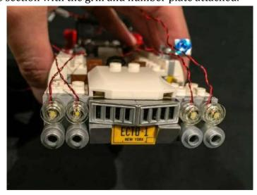
6.) Before reconnecting the white Lego pieces which make up the front bonnet, ensure that the cables from the LEDs are laid in between the studs of the Lego plates underneath as per below example images.
