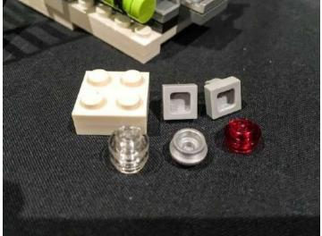
Take one of the provided grey Lego pieces with clip and place 1 standard Dot Light (non kashing) on top of the stud. Secure the LED in place by connecting the transparent red round piece over the top ensuring that the LED component part is facing the correct way up.
