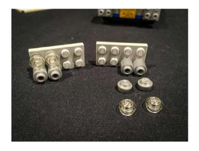
Take 1 standard Dot Light (non kashing) and place it on top of the stud of the grey round plate ensuring the LED component part is facing the correct way up. Secure the LED in place by connecting the transparent Lego plate over the top.
