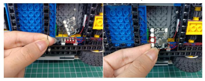
Connect the cable from the taillight to the D port.
