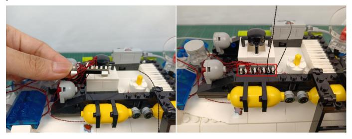
Tuck excess cables at the back of the expansion board with the tweezer.
