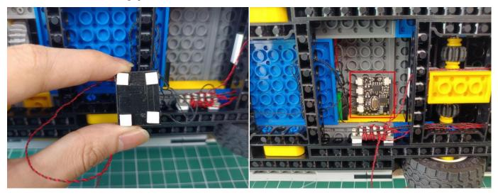
This completes installation of this LED Lighting Kit. ENJOY! (A port: headlights; B port: lights inside; C port: lights from the roof; D port: taillights.)
