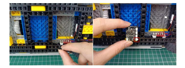
Connect the cable from the inside (the longer one) to the B port.
