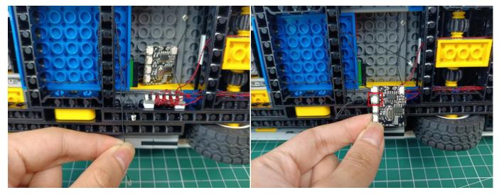
Connect the cable from the roof (the shorter one) to the C port.
