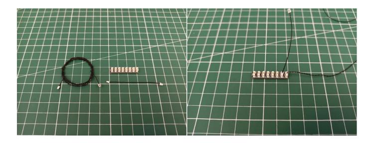
Take the following cables, connect them to the expansion board, tuck excess cables around the expansion board (except the cables from the blue piece).
