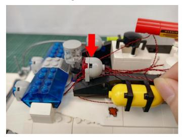
Take a  $50 \, \mathrm{cm}$  connecting cable, a  $5 \, \mathrm{cm}$  connecting cable, an  $8 - \mathrm{port}$  expansion board, assemble them as per below.
