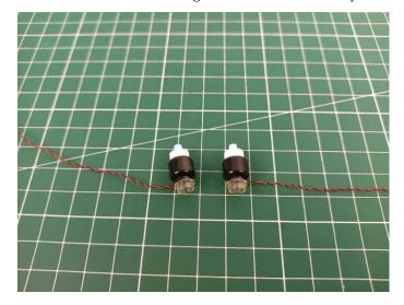
Thread the cable through the gray piece and reconnect the black piece.
