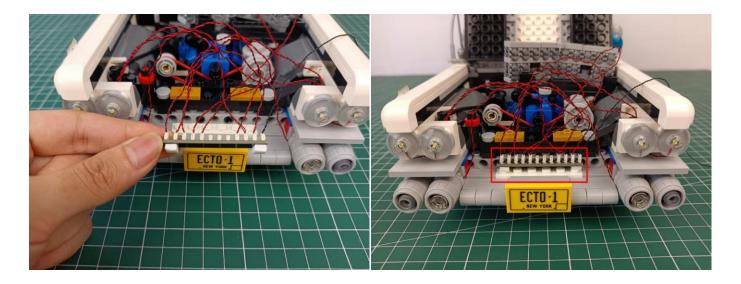
Thread the cable from the expansion board through the following hole, and pull it out from the bottom.
