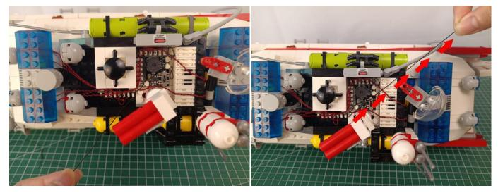
Continue to thread the cable through the following space, and pull it out from the back.
