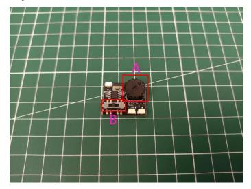
Connect the following 5cm cable from the expansion board to the power port on the Flicker Effects Board.
