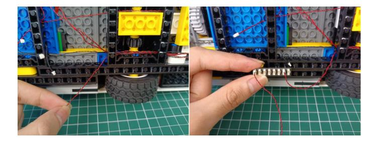
Connect the cables from the headlight to the expansion board.
