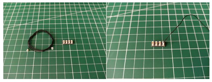
Connect all the cables from the roof to the expansion board.
