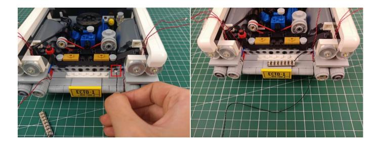
Connect all the cables from the head to the expansion board.
