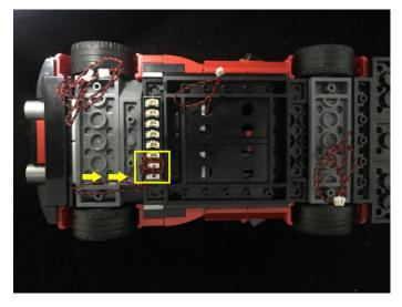
Connect the 2 cables at the other side of the tail to the expansion board.
