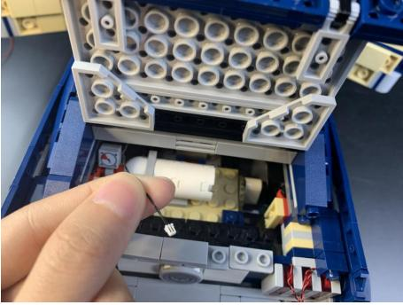
Take the 8-port Expansion Board. Stick adhesive squares to both sides. Connect the 15cm connecting cable to it
