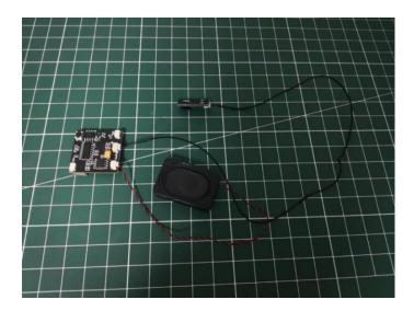
Connect the 5cm connecting cable from the expansion board to the OUT port on the Acousto-optic Control Switch Board.
