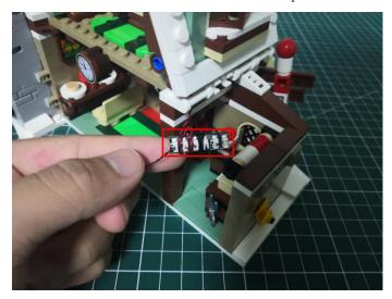
Take a 15cm connecting cable, connect it to the expansion board.
