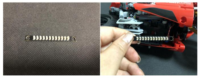
Stick the expansion board to the following place underneath the motorcycle with adhesive squares as per below.
