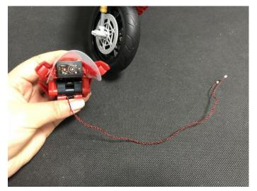
Thread the cables through the following space to the bottom of the motorcycle, reconnect the head of the motorcycle.
