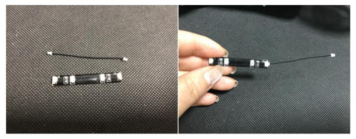
Stick the strip light next to the expansion board, connect the connecting cable to the expansion board, tuck excess cable as per below.
