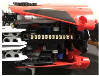
Take a blue strip light, a 5cm connecting cable, connect the connecting cable to the strip light.
