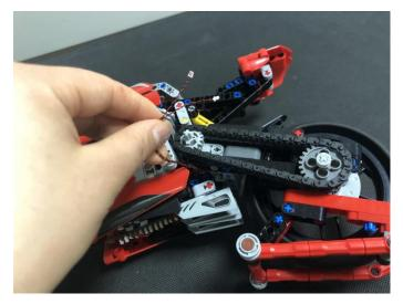
Thread the cables through the following space and connect them to the expansion board underneath.
