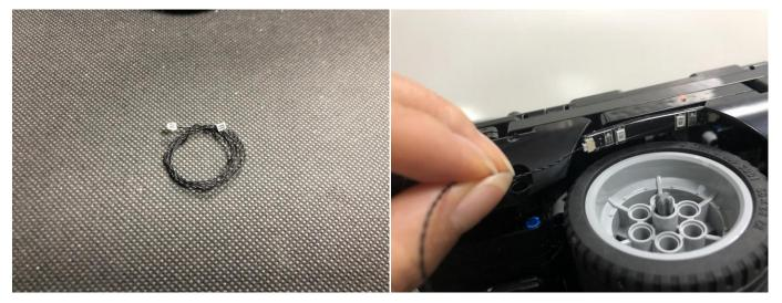
Turn the car over, thread the cable through the following space to the other side of the car, tuck excess cable as per below.
