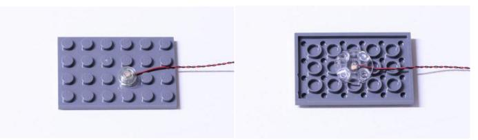
Place wires on the surface or under the building blocks.
