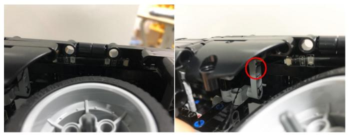
Thread the cable through the following spaces (note: you can thread the cable through any hole), and pull it backward.
