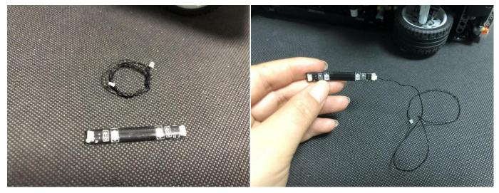
Stick the strip light to the following place over the front wheel. Thread the cable through the following space.
