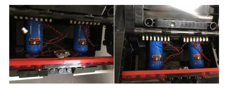
Take a blue strip light, a 30cm connecting cable, connect the connecting cable to the strip light.
