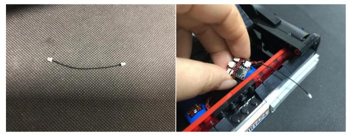
Stick the Flicker Effects Board to the following place, connect the cables on the Flicker Effects Board to the expansion board.
