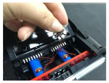
Take a 5cm connecting cable, connect it to the power port on the Flicker Effects Board.
