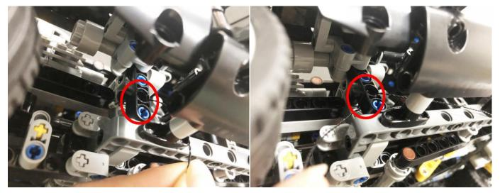
Remove the front tire, thread the cable through the following space.
