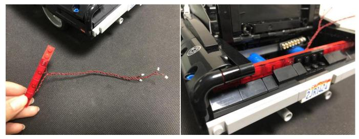
Connect the cables of the lights to the expansion board.
