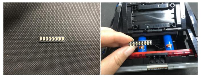
Stick the expansion board to the following place with adhesive squares, reconnect the tire, and the gray piece we removed before.
