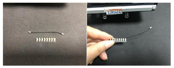
Connect the other end of the connecting cable to another expansion board, stick the expansion board to the following place with adhesive squares.
