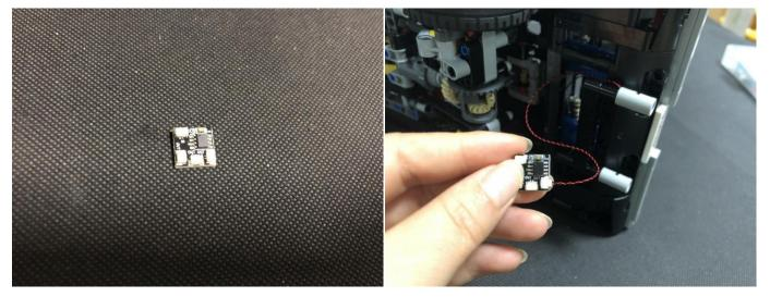
Take a red 15cm dot light, repeat the previous steps to install light for the other pipe, also connect the cable of the light to the Flicker Effects Board.
