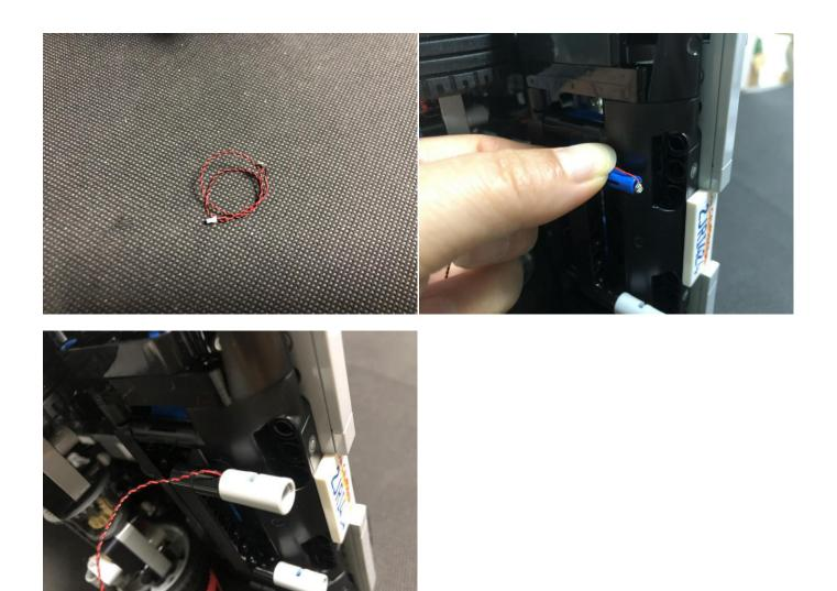
Take the Flicker Effects Board, connect the cable of the light to the Flicker Effects Board (note: do not connect it to the power port), as per below.
