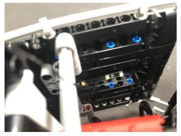
Thread the cable from the strip light through the following space, pull it out from the back.
