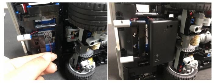
Connect the cable from the battery pack to the power port on the Remote Control Switch Board.
