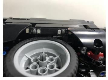
Take a 30cm connecting cable, connect it to the strip light over the back wheel.
