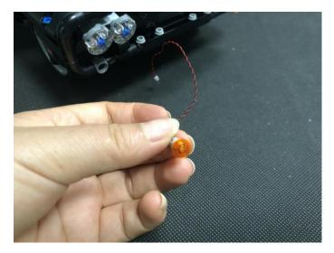
Thread the cable through the following hole, reconnect the light.
