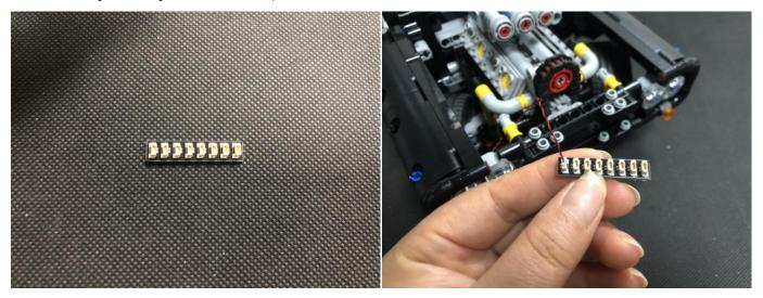
Tuck excess cable, stick the expansion board to the following place with adhesive squares.
