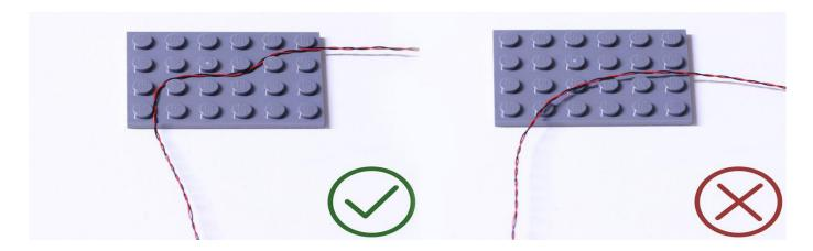
Be careful when insering the micro connector to the micro expansion board. With connecting cable side facing down, conenct the connector to the board as per below. In case of damaging the pieces, do ont force to connect the pieces.
