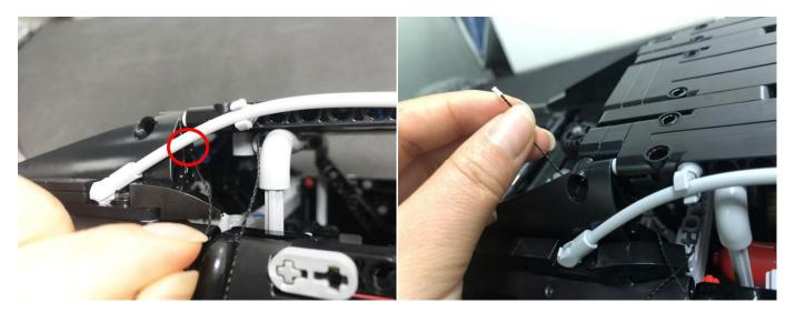
Thread the cable through the following space to the bottom of the car.
