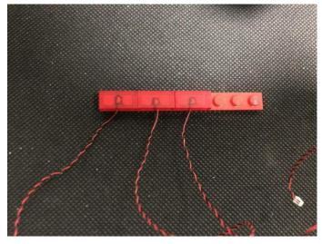
Place the last light on the stud, secure the light with the trans red 1x1 plate.
