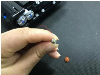
Secure the light with the trans orange plate.
