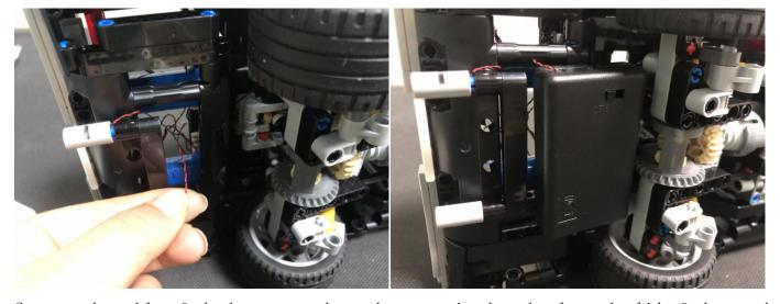
Connect the cable of the battery pack to the expansion board, close the lid of the trunk.
