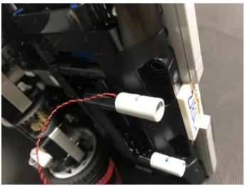
Take the Flicker Effects Board, connect the cable of the light to the Flicker Effects Board (note: do not connect it to the power port), as per below.
