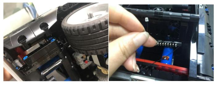
Tuck excess cable before connect the connecting cable to the expansion board.
