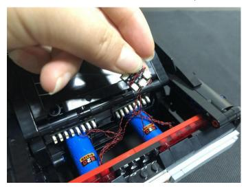
Take a 5cm connecting cable, connect it to the power port on the Flicker Effects Board.
