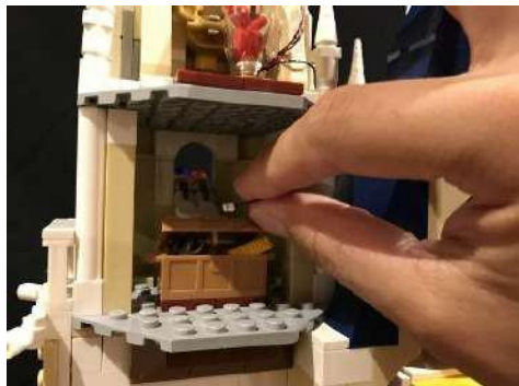
Take the 15cm cable from the expansion board and then loop it behind and then thread through the right side window as per below
