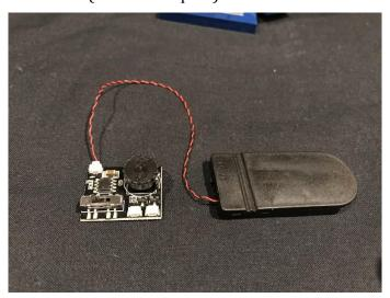
Connect the Dot Light cable from the roof to one of the output ports of the Multi-Effects Board. Turn the channel far left for the "pulse" effect and then turn on the battery pack. Adjust the speed of the effect by turning the wheel either clockwise or anticlockwise.
