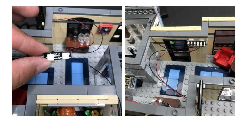
36.) Take the roof directly above the building and then connect the Flashing White 30cm Dot Light cable as well as the 15cm Connecting cable from the strip light to the spare ports on the 6-port expansion board.
