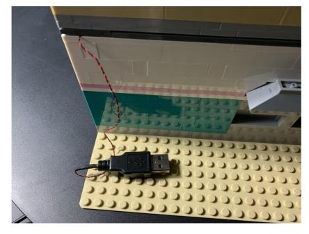
Connect the power supply and ensure the lights we have installed so far are working OK.
