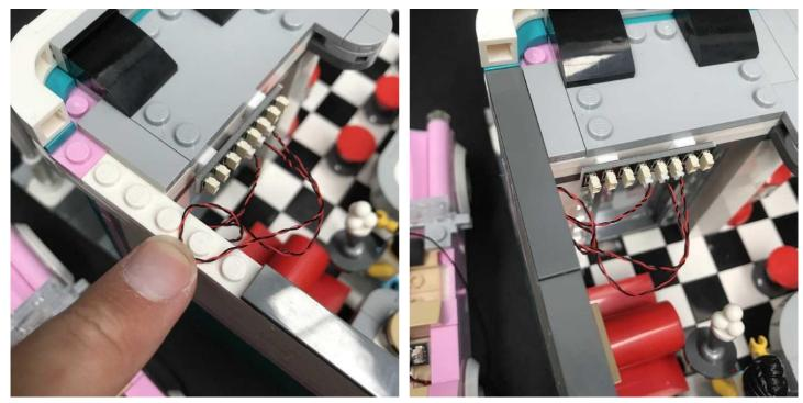
4) Take Take the USB cable and then place it behind the Downtown Diner as per below. Bring the cable over the wall and then connect it to a spare port on the 8-port Expansion Board.
