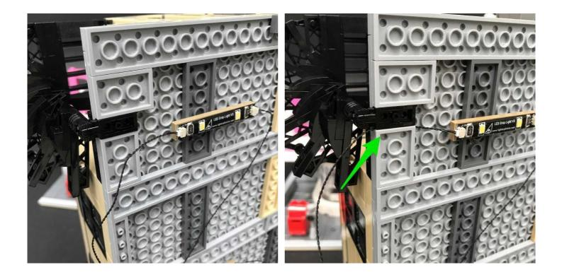
Secure the 15cm Connecting Cable that connects the two strip lights underneath the 2x6 plate. Securing these connecting cables will also prevent them from dangling down and being seen from the outside looking in.
