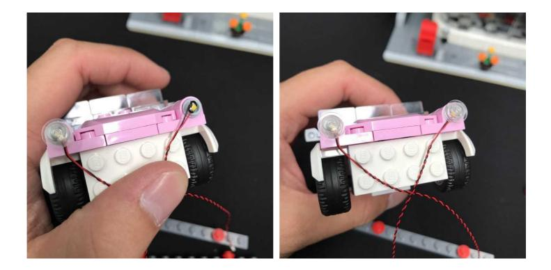
3.) Lay both Dot Light cables down the side of the White 2x4 plate and then reconnect the front bumper section over the top.
