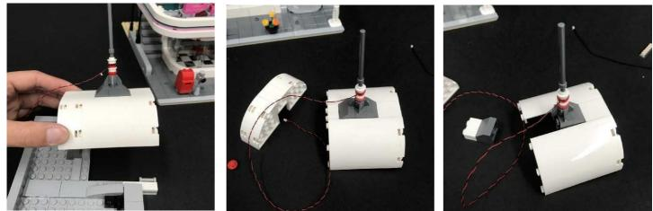
Lay the cable down in between studs and then reconnect the middle section over the top of the cable (ensuring the cable is laid in between studs). Reconnect the back section.
