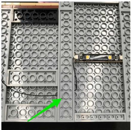
Take the 30cm Connecting cable and then secure it underneath the 2x6 plate at the bottom as per below:
