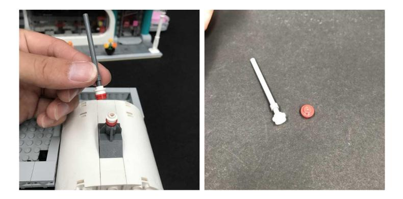
Take the remaining Flashing White 30cm Dot Light and place it on top of the white round stud on the roof ensuing the cable is facing toward the back. Secure the Dot Light in place by connecting a provided Trans Red round plate in lieu of the original red round plate.
