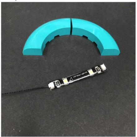
Place the two arc pieces together and then using the adhesive backing, stick the strip light underneath ensuring the strip light is stuck directly on the centre of thetwo pieces.
