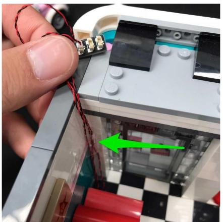
Using 2x Adhesive Squares, mount the expansion board to the inside of the diner in the following position.
