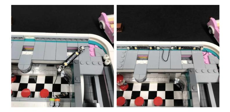
15.) Reconnect the two sections of the Diner sign and then turn the battery pack on to test and confirm the lights we have installed so far are working OK.
