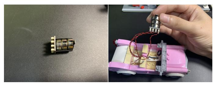
Secure the power supply to the rear seat, taking care that the power switch is facing up
