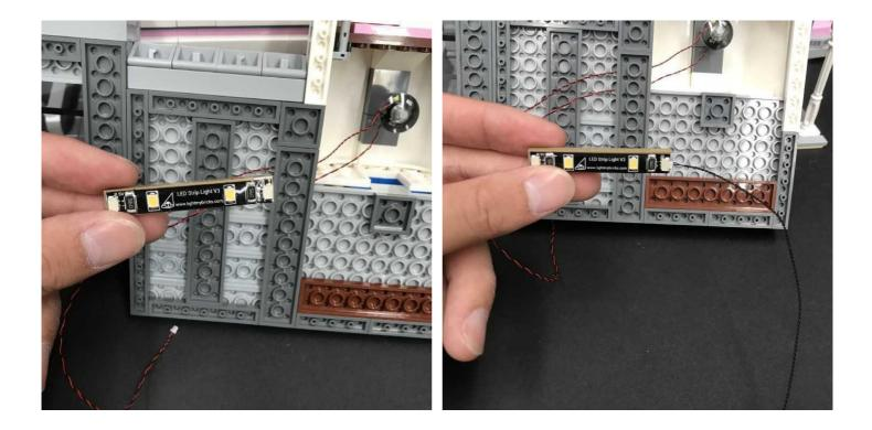
Connect the other end of the White 15cm Dot Light to the left port on the strip light and then mount the strip light to the bottom of the roof in the following position:
