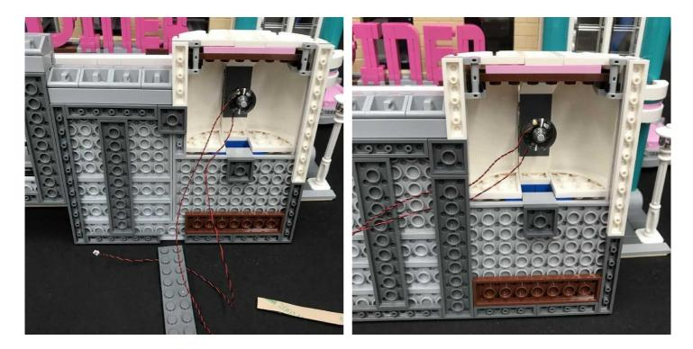
33.) Take the remaining White Strip Light and stick it to the remaining LEGO plate 1x6. Connect the last 15cm Connecting Cable to the right port on the strip light.
