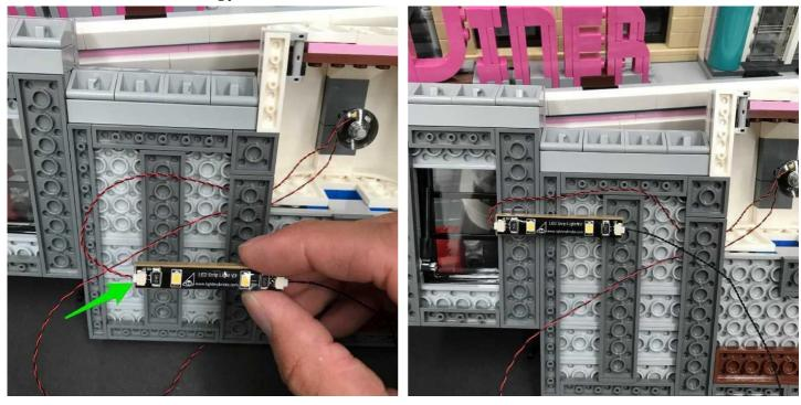
34.) Take the 6-port Expansion Board and then to the spare ports, the connect the 30cm connecting cable from the third koor, the lamp post cable from second koor, and the 15cm connecting cable from the strip light on the front arc.
