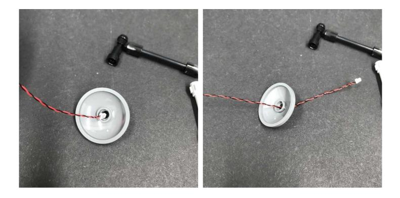
Place the other end of the Dot Light inside the bottom of the trans clear minifigure head and then from the top of the dish, pull the cable all the way up and then reconnect the two together. This should secure the dot light in place and look similar to below:
