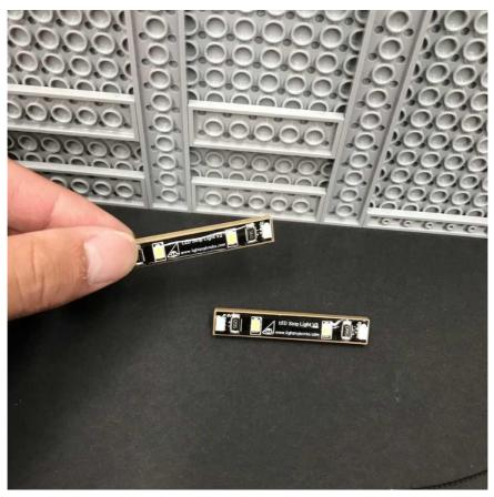
Connect the two strip lights together using a 15cm Connecting Cable and then connect another 30cm Connecting Cable to the end of one of the strip lights.
