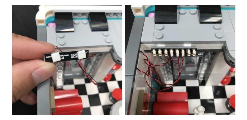
3.) To prevent cables from dangling down you can secure them underneath the top tiles by laying them in between studs.
