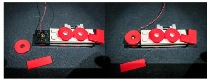
Take another 2 flashing dot lights and repeat the same step for the 2x letter "O"'s ensuring the LED component part is laid in between the 4x Lego studs and visible in the center.
