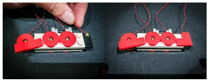
Ensure all cables for the flashing LEDs are facing up toward the handle
