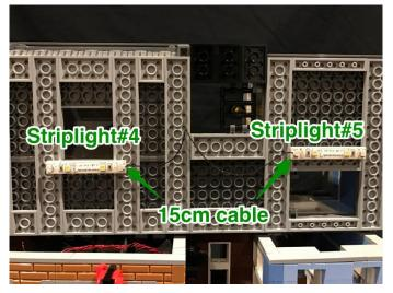
40.) Connect the 2 strip lights we just installed to the rest of the lighting circuit by connecting the other end of the 15cm cable from the 12-port expansion board to striplight#4
