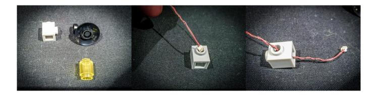
Then thread the cable from the connector side up through the smaller hole of the transparent yellow Lego piece. Thread this all the way until the dot light part is up against the Lego piece.
