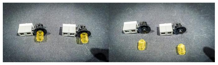
Take one of the dot lights and thread the cable from the connector side up through the smaller hole of the transparent yellow Lego piece. Thread this all the way until the dot light part is up against the Lego piece.
