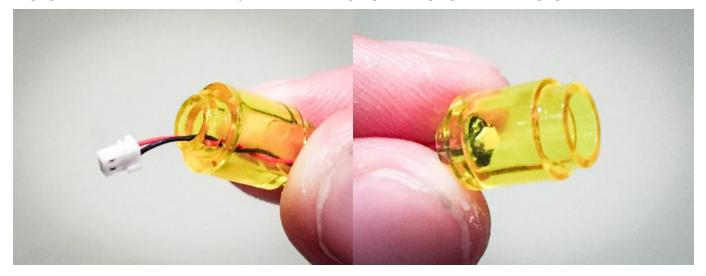
Reconnect the black lamp shade piece on top of the transparent yellow piece and then connect the black lamp shade piece back to the grey piece.
