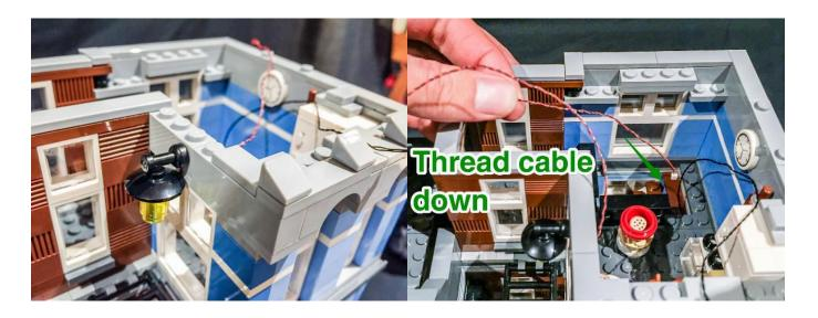
45.) Lift and flip over the entire 3rd level on it's side so that we can pull the cable from the lamp down from the spacing and then connect this to a spare port on the 6-port expansion board.
