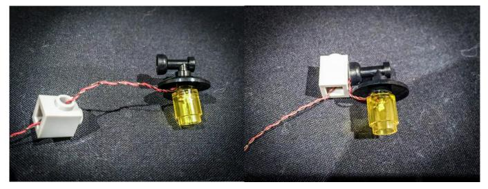
44.) Reconnect the lamp section back to its original position and then thread the cable from the lamp down the staircase section as we will need to connect this to the 6-port expansion board on level 2.
