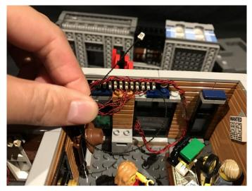
39.) Take 2x LED strip lights and then stick/connect them on the ceiling of level 2 (underneath the top level) in the following position. We will refer to them as striplight#4 and striplight#5. Connect striplight#4 and 5 together using another 15cm connecting cable.
