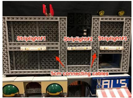
18.) Take a 15cm cable that we connected earlier to the expansion board and connect the other end of this to the left port of striplight#1.
