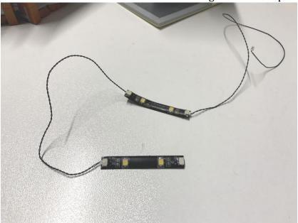
Connect the 30cm connecting cable we thread to the second floor before to the left port of the strip. Connect the strips to the third floor as we did before. Thread the 30cm connecting cable through to the third floor
