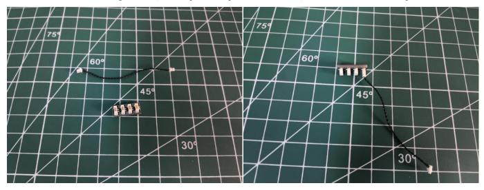
Connect the cables to the expansion board, tuck excess cables around the expansion board.
