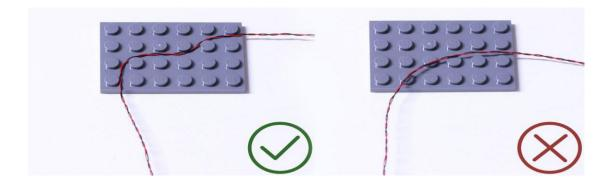
Insert the connectors to the ports.
