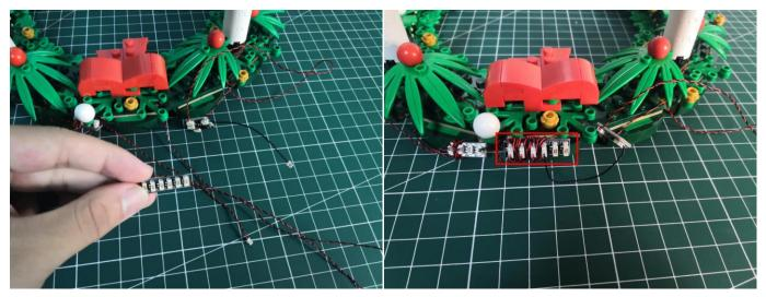
Take the Round Coin Cell Battery Pack, connect it to the expansion board.
