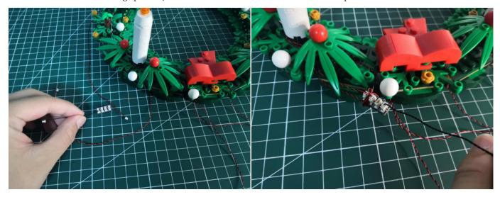
Take a 5cm connecting cable, a Flicker Effects Board, connect the connecting cable to the IN port on the Flicker Effects Board.
