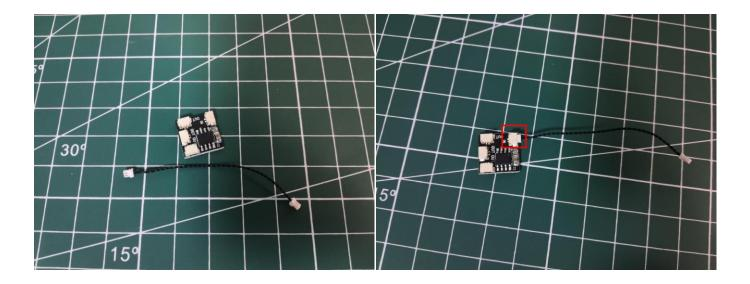
Connect the cable from the expansion board to the OUT port on the Flicker Effects Board.
