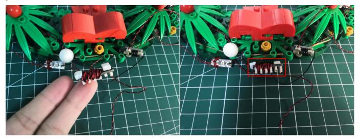
Stick an adhesive square to the back of the 4-port expansion board, secure it to the following place.
