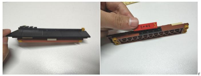
econnect the brown piece, pull the cable upward, reconnect the piece with characters to secure the cable
