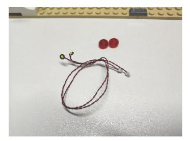
With lighting side facing up, install the Dot Lights to the following places at the roof, secure them in place by connecting the red pieces over. Hide the cables underneath in between studs before reconnecting the roof
