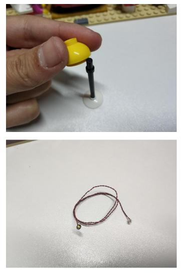
tie the light at the top of the lamp post, wind the cable around the post
