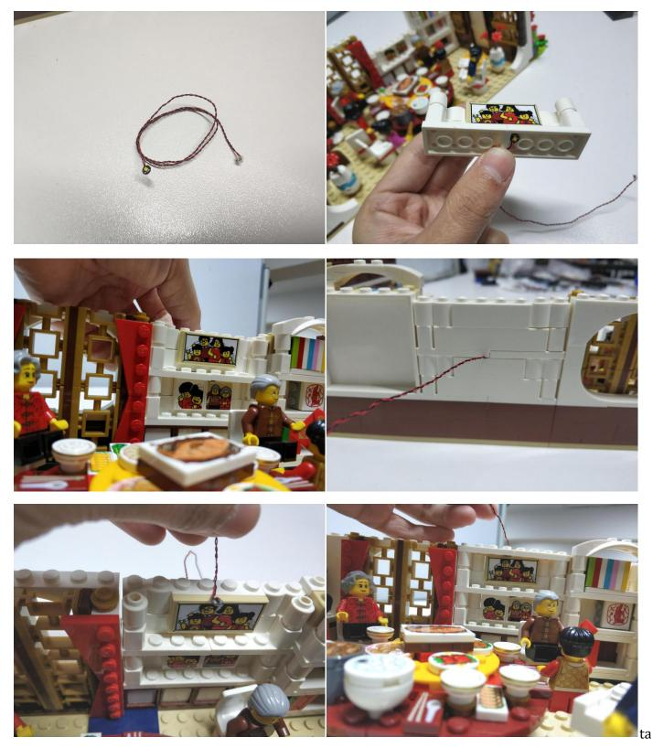
ke a warm white 15cm Dot Light, place it at the middle of the door, reconnect the pieces over the door, pull the cable to the back of the pieces
