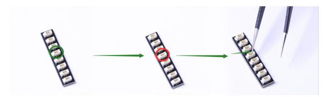
When installing dot lights, make sure they are correctly placed (Yellow LED package is exposed). You can put they either on the top of the studs or between studs.
