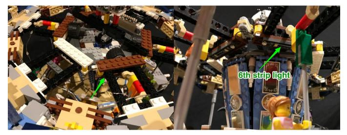
After finishing installing all 6 strip lights, connect the cable of the battery pack to the expansion board, then turn on the power to test if all the lights are working OK
