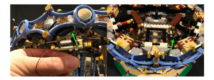
Connect all 4 cables to the next available ports on the 12-port Expansion board.
