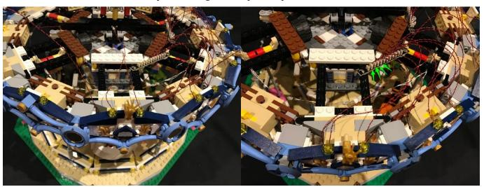
20.) Take a **15cm Connecting Cable** and then connect it to the remaining port on the 12 port expansion board. Connect the other end of the cable to a new **12 Port Expansion board** then mount the expansion board to the following position using 2x **adhesive squares**.
