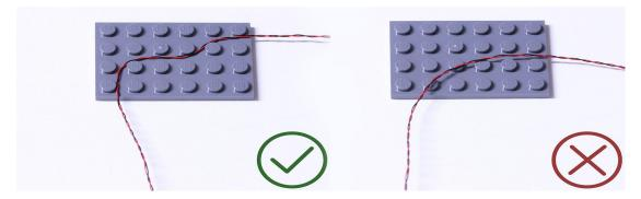
Insert the connectors to the ports.
