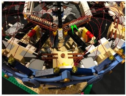
Then connect the remaining 10x Dot Light cables to the last 12-port expansion board.
