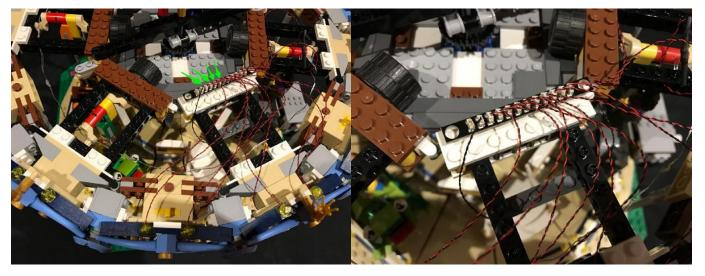
Test that all lights are working OK by connecting back your Battery Pack (or USB cable) to a spare port on the expansion board.
