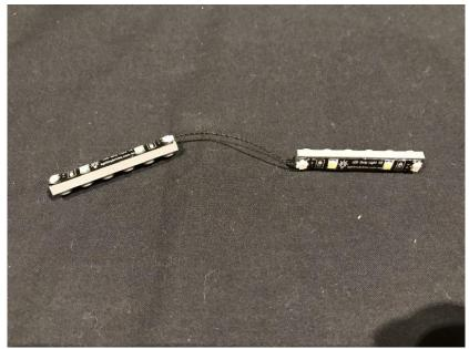
Continue this process to connect **6x White Strip Lights** (using total of five **5cm connecting cables**)
