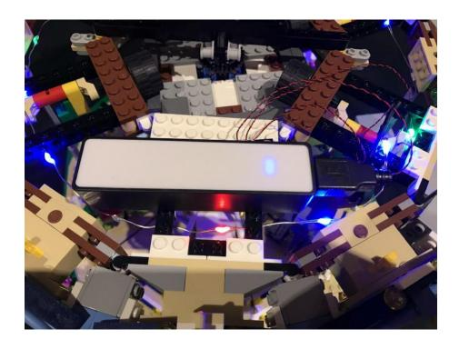
7.) Take a **White Strip Light** and then carefully peel off the adhesive backing to allow you to stick onto the base of a provided **LEGO 1x6 Plate**. Connect a **5cm Connecting Cable** to the right port.
