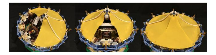
Locate where the Battery Pack/USB power cable are and then lift up the flap. Connect up the power bank/AA Battery Pack and place inside before reconnecting the top centre flag piece and remaining white pole sections.
