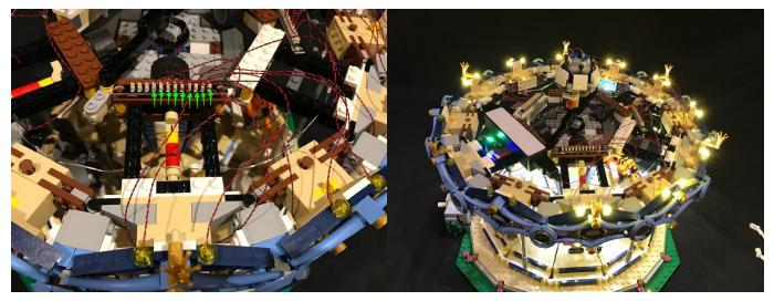
22.) Take a **5cm Connecting Cable** and then connect it to the far left port on the 12 port expansion board. Connect the other end of the cable to the last remaining **12 Port Expansion board** then mount the expansion board to the following position using 2x **adhesive squares**.
