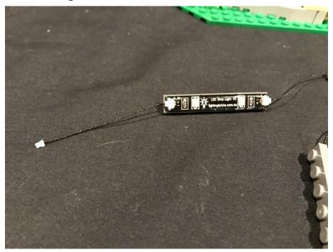
8.) Take all 6 Strip Lights over the top of the Carousel and then connect the other end of the 5cm connecting cable to the port on the expansion board second from the left.
