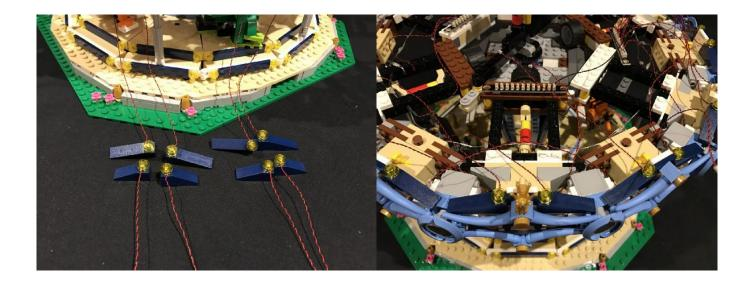
Connect all 8 Dot Light cables to the first remaining ports on the new 12-port Expansion Board and then test that all lights are working OK by connecting back your Battery Pack (or USB cable) to a spare port on the expansion board.
