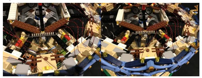
16.) Take a **5cm Connecting Cable** and connect it to the far left port on the expansion board and then connect the other end to a new **12-port Expansion Board** and then mount to the following position using another 2x **adhesive squares.**
