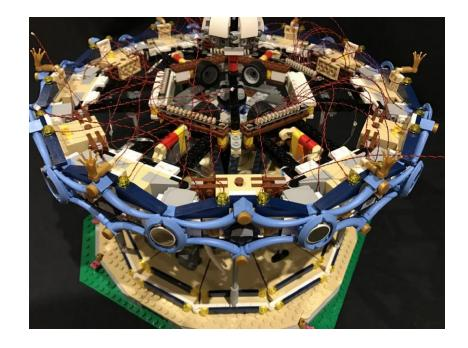
First connect the 2 lights from the right section (top and bottom) to the remaining 2 ports on the 12-port expansion board towards the right.
