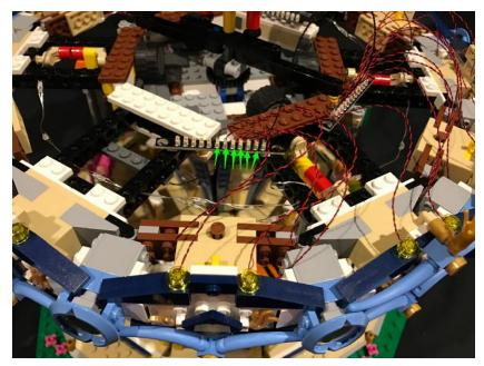
Test that all lights are working OK by connecting back your Battery Pack (or USB cable) to a spare port on the expansion board.
