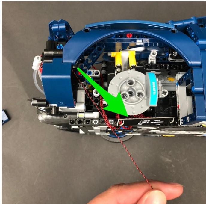
Flip the Bugatti back over and hide the cable behind the light grey piece as per below.
