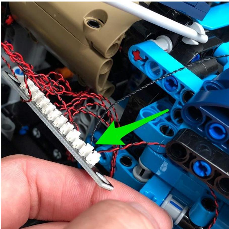
Neatly push the expansion board and cables into the passenger foot area before seating the Battery Pack over the top then thread the connecting cable down the space which leads to underneath the
