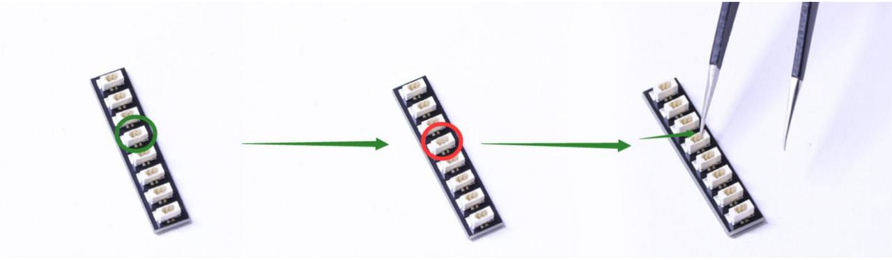
When installing dot lights, make sure they are correctly placed (Yellow LED package is exposed). You can put them either on the top of the studs or between studs.
