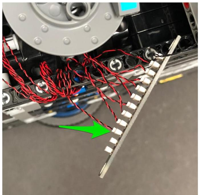
27.) Pull the expansion board down over the black technic brick to tighten all the cables then roll the expansion board up so the remaining excess cables wind around it. Tuck the expansion board into the space right under the disc brakes as per below.
