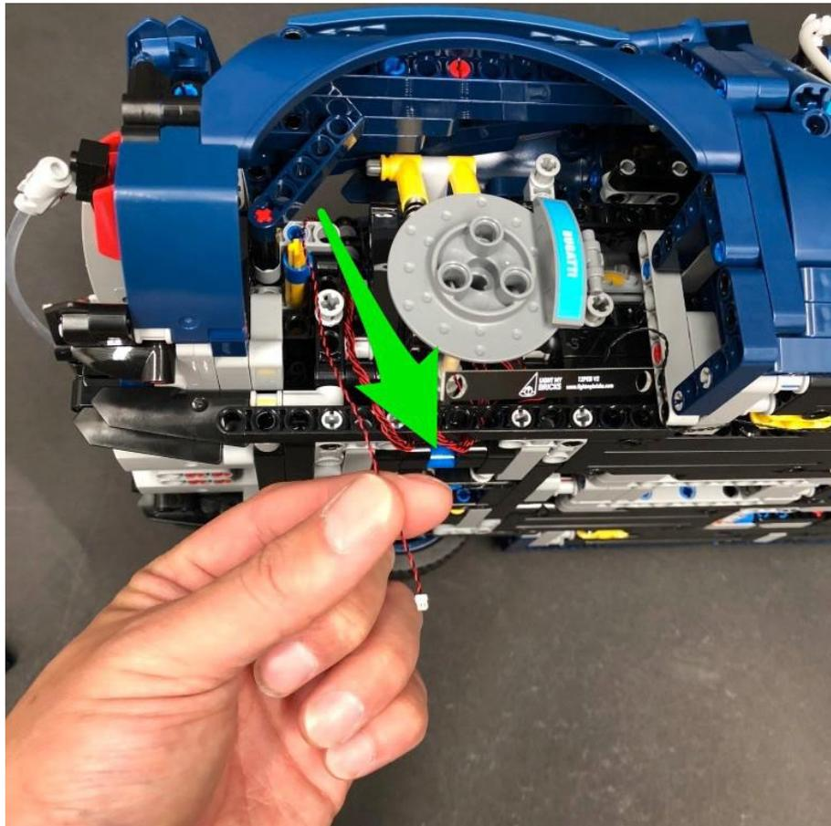
Loop the cable around the black technic brick (same way we did for the larger cable) before connecting it to the next available port on the 12-port Expansion Board.
