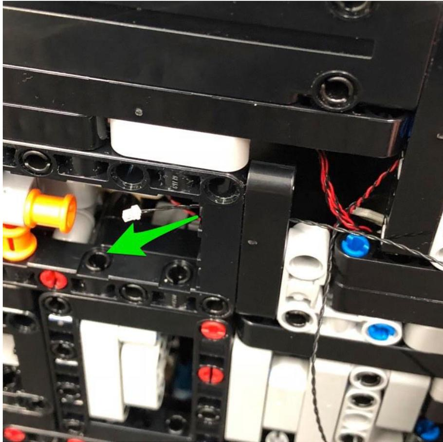
15.) Pull the cable all the way out toward the back and then thread it through the hole of the following light grey technic brick
