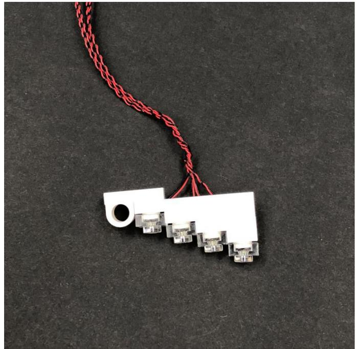
Continue to twist the cables around each other all the way to the end so that it forms one larger cable.
