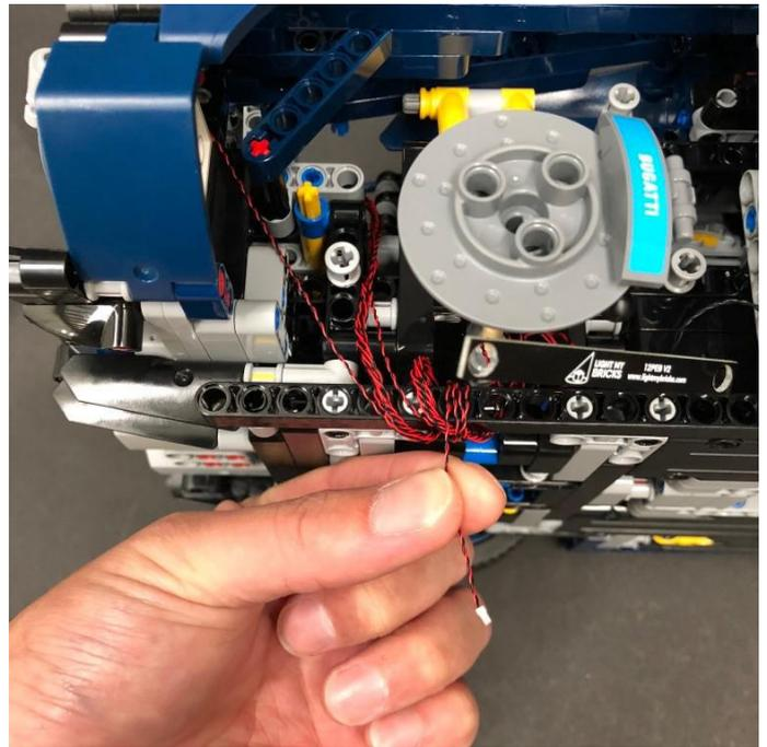
Connect the cable to the next available port on the expansion board.
