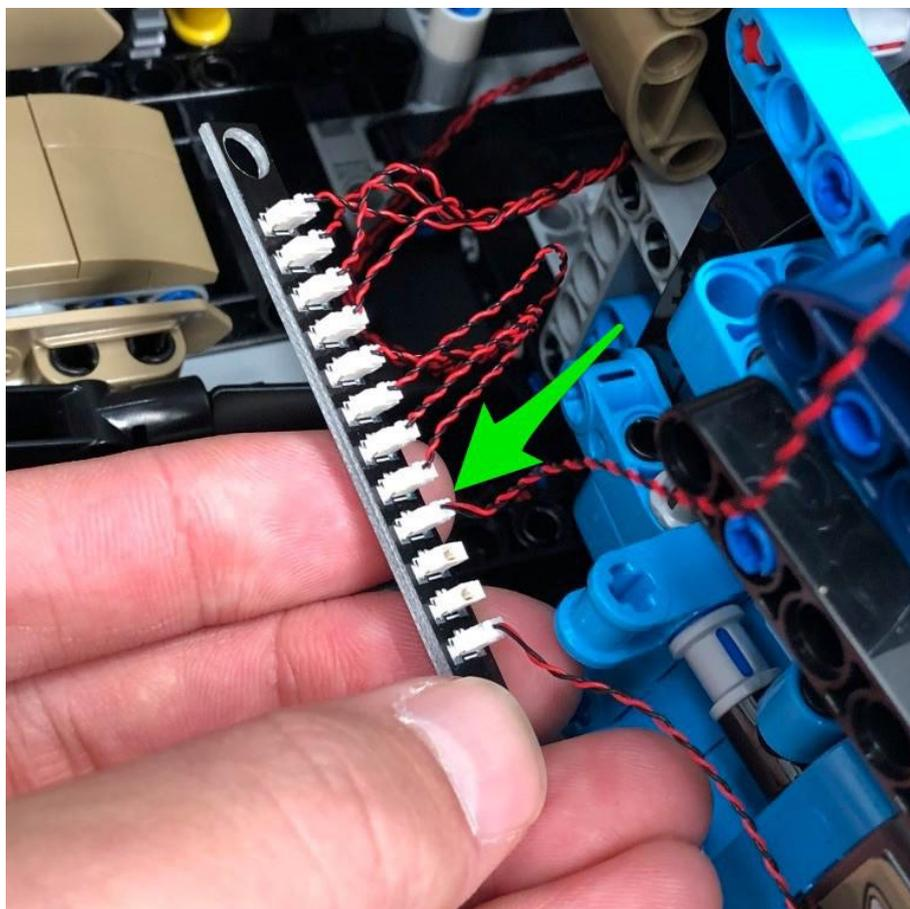
Eliminate excess cable from the light bar by folding the cable over twice and then twisting it around each other a few times as per below.
