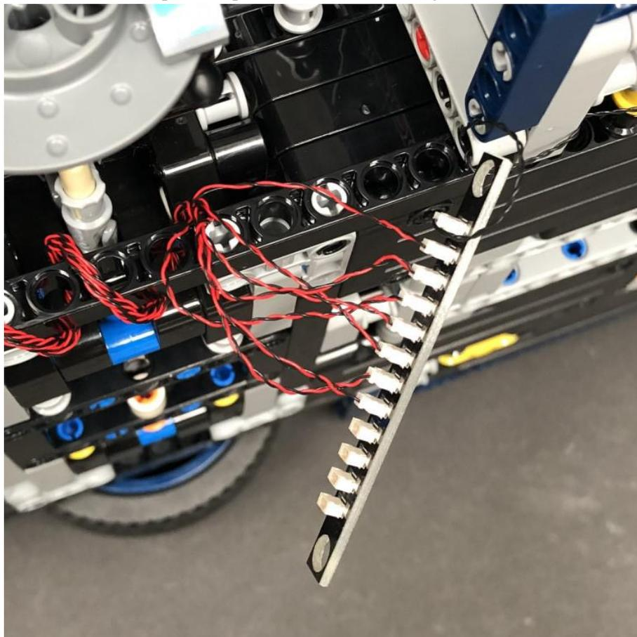
Turn the Bugatti back over and then ensure that the cables from the back of the spoiler are pushed flat so that the spoiler can easily come up and down without the wires getting caught.
