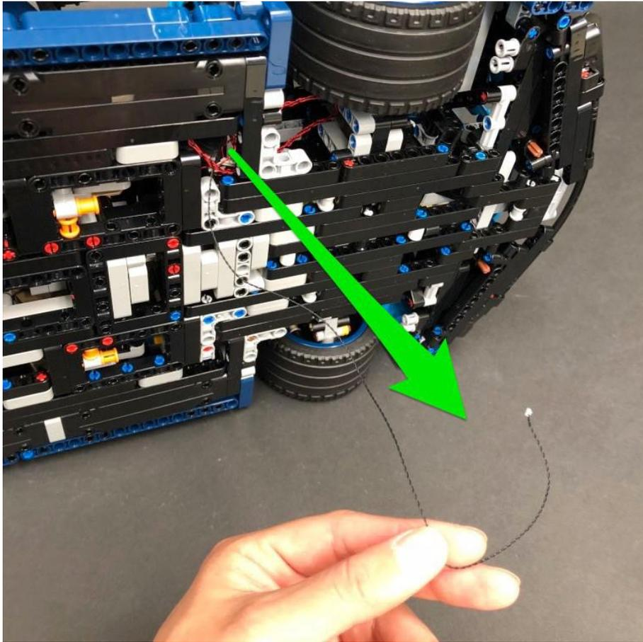
Thread the cable through the hole of the following black technic brick underneath the vehicle.
