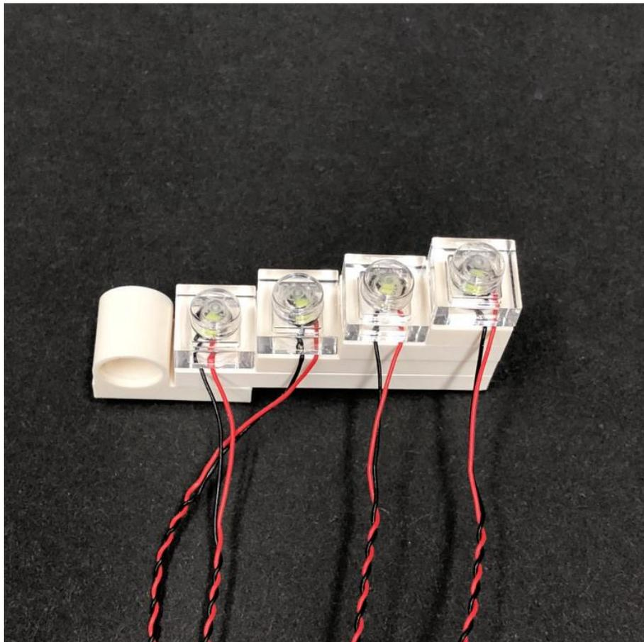
4.) Turn the headlight section over so that it is facing forward. Group all the cables together and twist them around each other.
