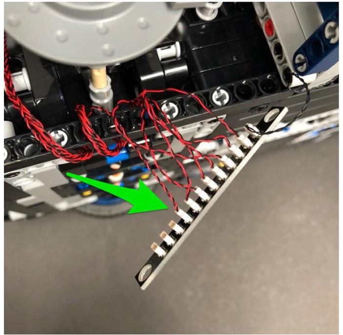
25.) Flip the Bugatti back over and then reconnect the right side of the red light bar. Thread the cable up the space above that leads to the back wheel then turn the Bugatti onto it's side to pull the cable out
