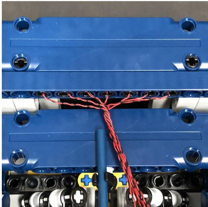
Continue to twist all the cables around each other all the way to the end to form one larger cable.
