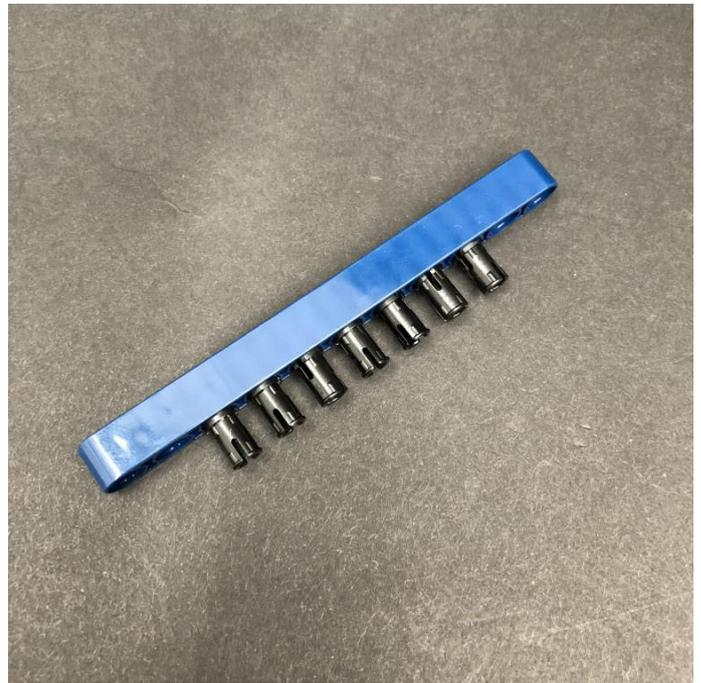
19.) Take a Red 30cm Dot Light and thread the connector end of the cable through the first technic pin. Thread it all the way through and then slightly bend the Dot Light on a 90 degree angle before pushing it inside the technic pin.
