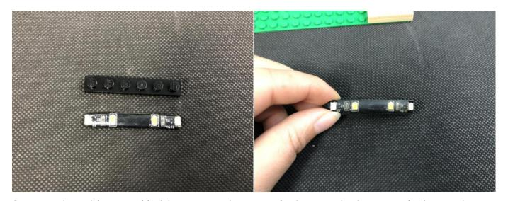
Connect the cable we pulled before to the strip light, stick the strip light to the roof.
