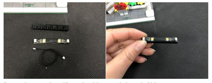
Connect the connecting cable to the right port of the strip light.
