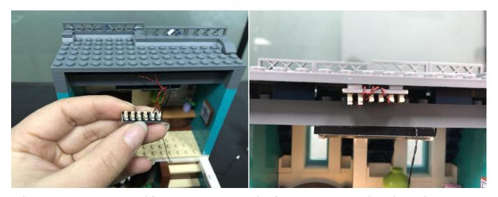
Take a 5cm connecting cable, connect it to the 6-port expansion board at the roof.
