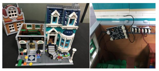
Take two 15cm connecting cable, a warm white strip light, a 1x6 black plate, stick the strip light to the plate.
