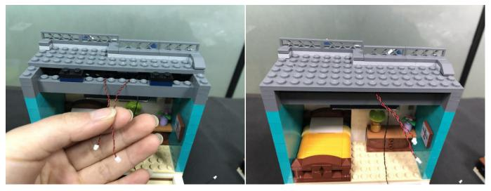
Connect the cables to the expansion board, stick the expansion board to the roof with adhesive squares.
