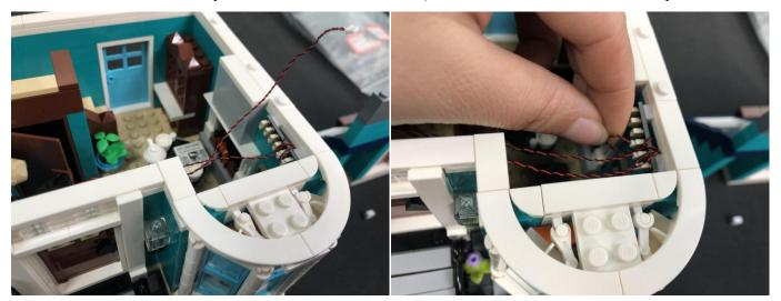
Take a 30cm connecting cable, connect it to the expansion board.
