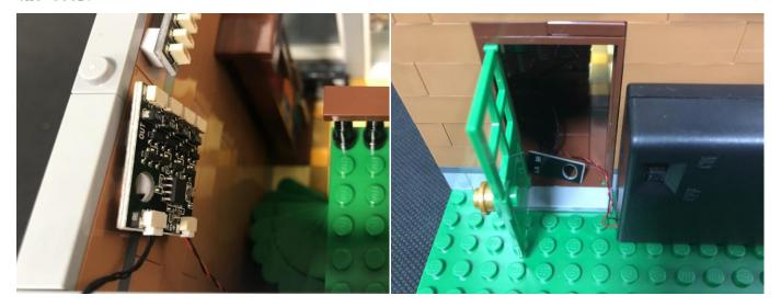
Take a 5cm connecting cable, connect the expansion board and the remote control switch board together.
