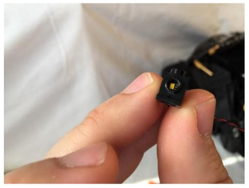
The Dot Light goes in through the back of the Headlight Brick. We want to make sure that the yellow LED element is facing the front for the best lighting effect.
