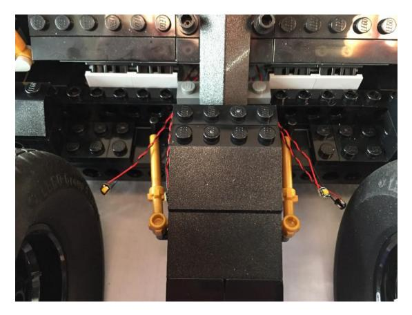
Push the wires through leaving a few cm of wire outside the vehicle.
