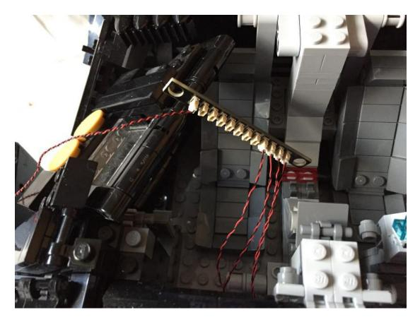
Connect the battery pack to the 12 Port Expansion board as well and turn it on.
