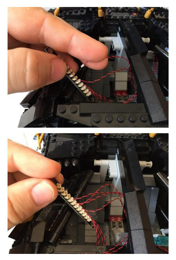
Connect the four dot lights that we have just fitted to the 12 port expansion board.
