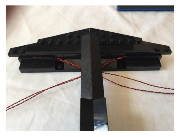
Repeat fitting dot lights to both sides. Try and keep the wires down so that they come out where the side of the panel is, rather than the top.
