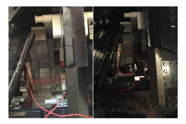
Push the 12 port expansion board down beside the seat. Rest the battery pack on the seat and turn it on.
