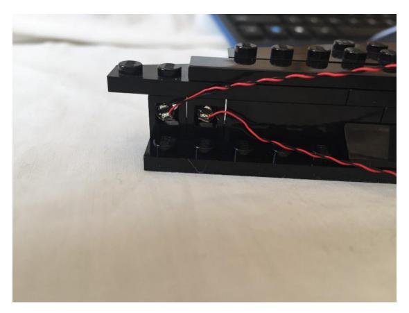
Once you have two dot lights resting in position, grab the 1 x 4 panel and reattach it so that it holds the dot lights in position.
