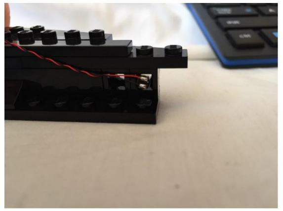
Now that the back of the headlight bricks are visible, we can fit the dot lights. As we did before, we want the LED sitting inside the headlight brick with the yellow element facing the front.
