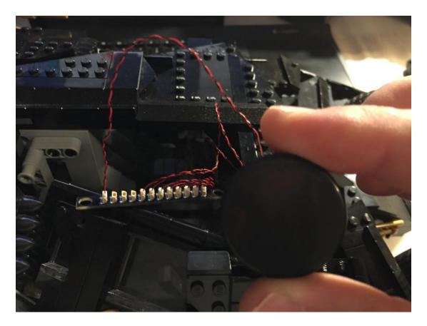
Connect the battery pack to the 12 port expansion board.
