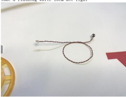
With lighting part facing down, connect the light to the hole at the center of the disc. Note: do not thread it through.
