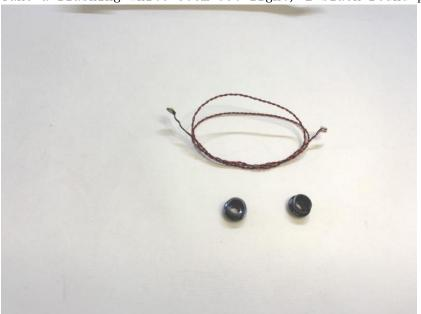
Thread the connector of the light through the hole, pull till the light is facing up, connect the other round plate over
